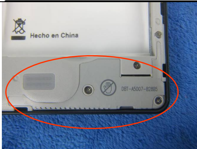
GSM/PCS/UMTS-FDD Antenna View
