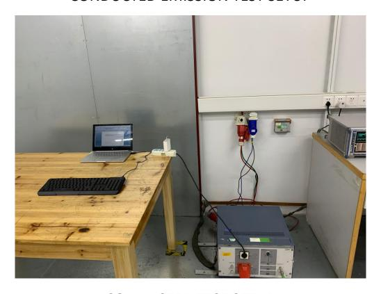
**CONDUCTED TEST SETUP**
