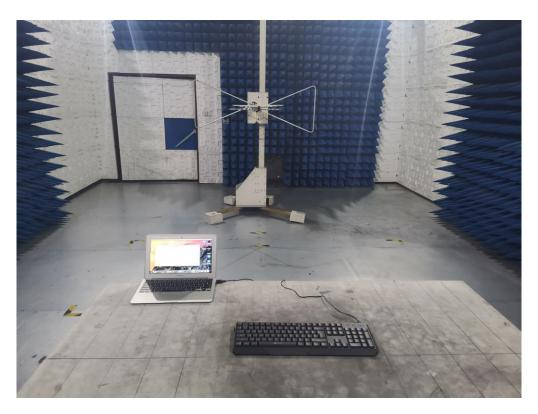
FCC RADIATED EMISSION TEST SETUP ABOVE 1GHZ
