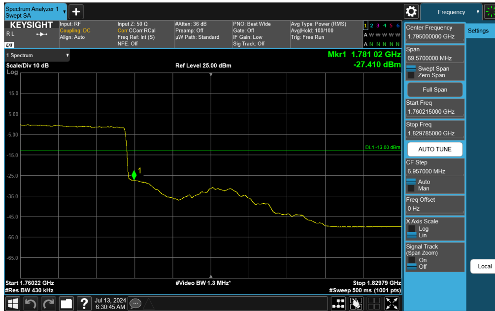
Plot 7-342. Upper Band Edge Plot (NR Band n66 – 40.0MHz DFT-s-OFDM \pi/2 BPSK - Full RB)
