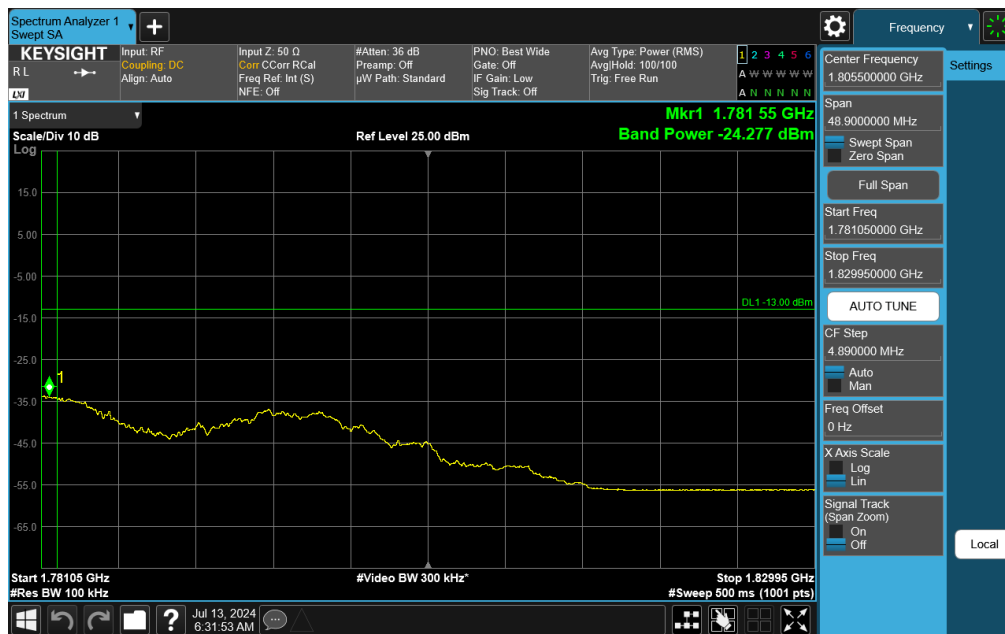
Plot 7-343. Upper Extended Band Edge Plot (NR Band n66 – 40.0MHz DFT-s-OFDM \pi/2 BPSK - Full RB)
