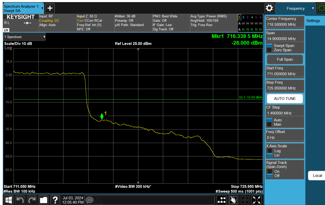
Plot 7-367. Upper Band Edge Plot (NR Band n12 – 10.0MHz DFT-s-OFDM QPSK- Full RB)
