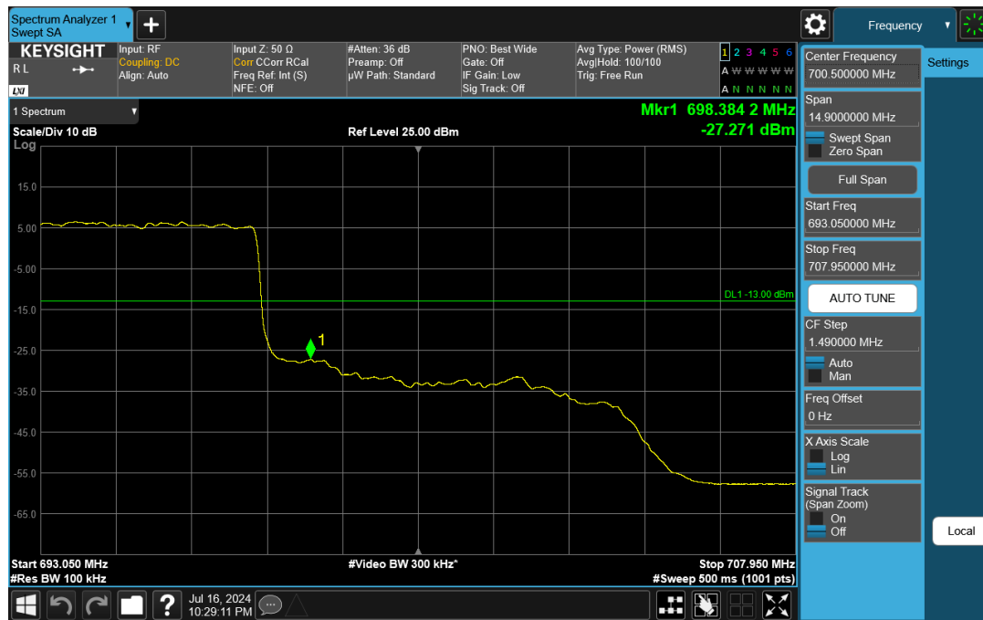
Plot 7-359. Upper Band Edge Plot (NR Band n71 – 10.0MHz DFT-s-OFDM QPSK - Full RB)
