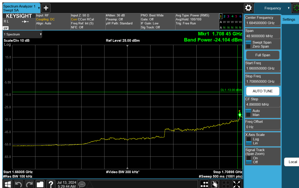
Plot 7-325. Lower Extended Band Edge Plot (NR Band n66 – 20.0MHz DFT-s-OFDM QPSK - Full RB)
