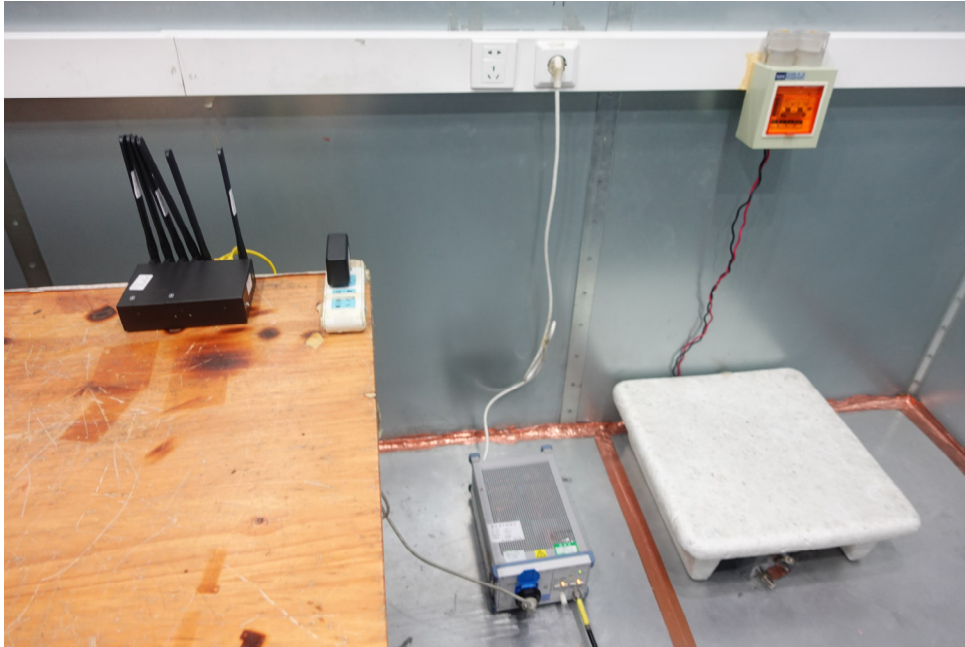
Picture 2: Conducted Emissions Test Setup
