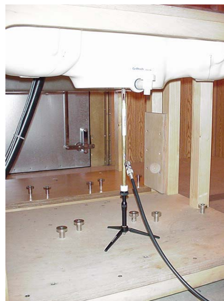
2450MHz Dipole Setup
