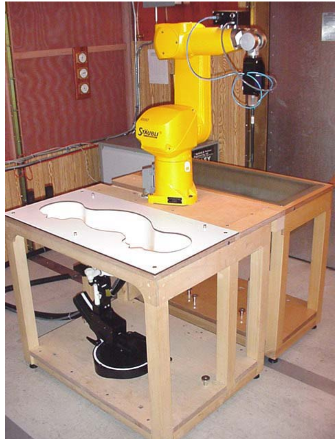
DASY4 SAR Measurement System with SAM phantom
