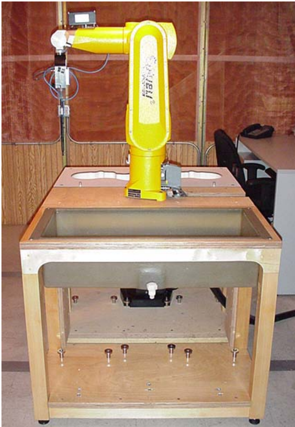
DASY4 SAR Measurement System with planar phantom
