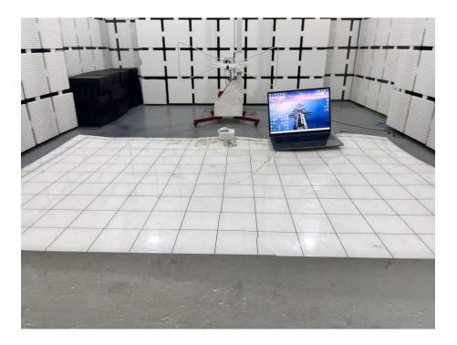
Set-up for Radiated Spurious Emission, Above 1GHz
