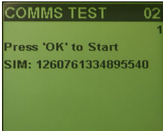
The bottom row of each screen displays information being transmitted / received. If at any point *Connected* is NOT shown on the LCD, or *Error* appears on the LCD, the meter is likely experiencing a communication error, due to a faulty communication module or a network error. In either case, ensure the meter receives a strong wireless signal before attempting the communications test again.
