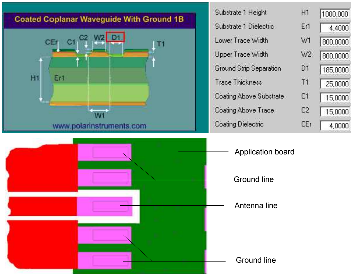
Figure 13: Micro-Stripline on 1.0mm standard FR4 2-layer PCB - example 1
