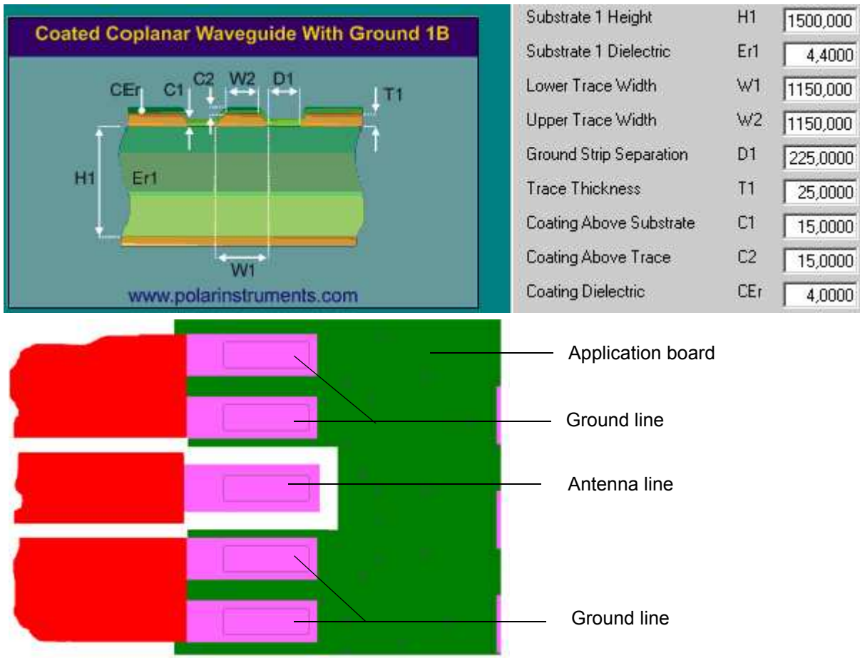
Figure 16: Micro-Stripline on 1.5mm Standard FR4 PCB - example 2
