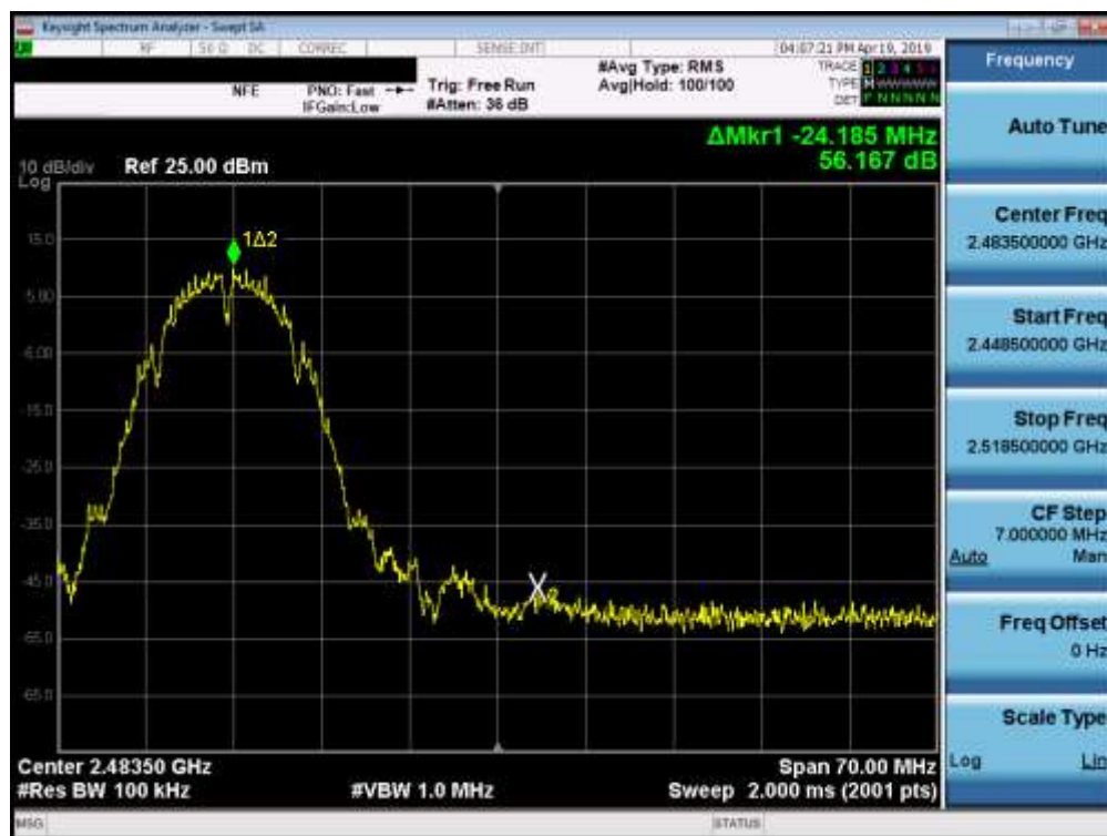
Plot 7-22. Band Edge Plot (802.11b – Ch. 11)
