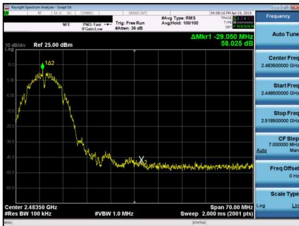
Plot 7-21. Band Edge Plot (802.11b – Ch. 10)
