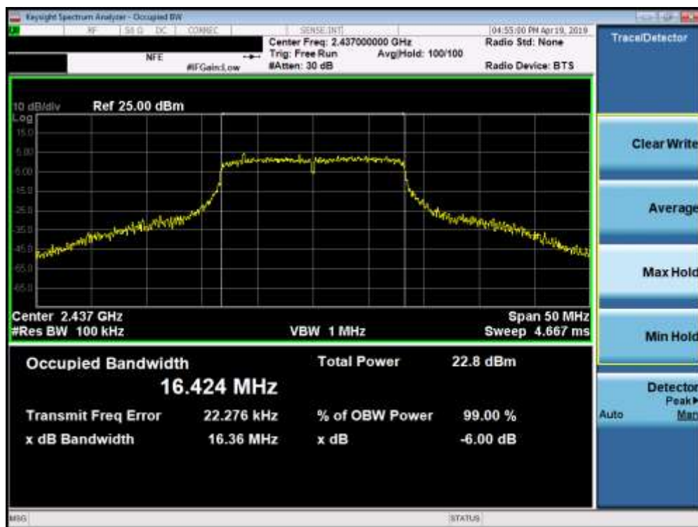
Plot 7-5. 6dB Bandwidth Plot (802.11g – Ch. 6)
