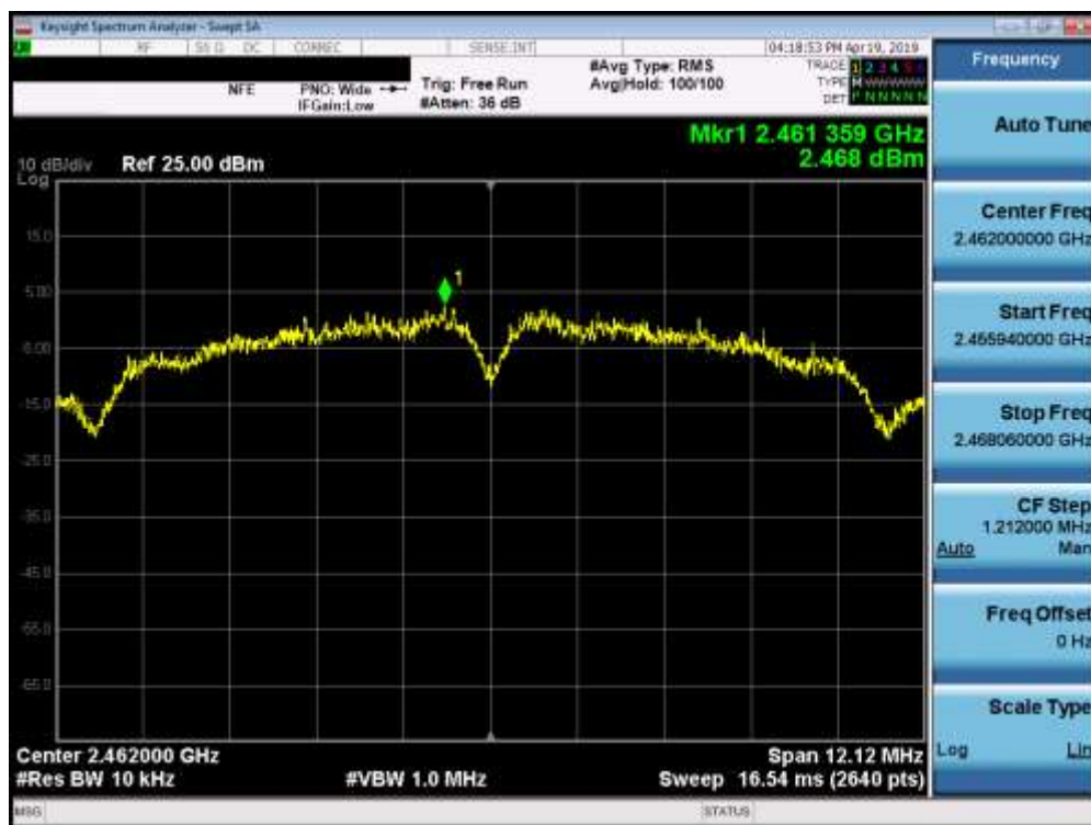
Plot 7-12. Power Spectral Density Plot (802.11b – Ch. 11)
