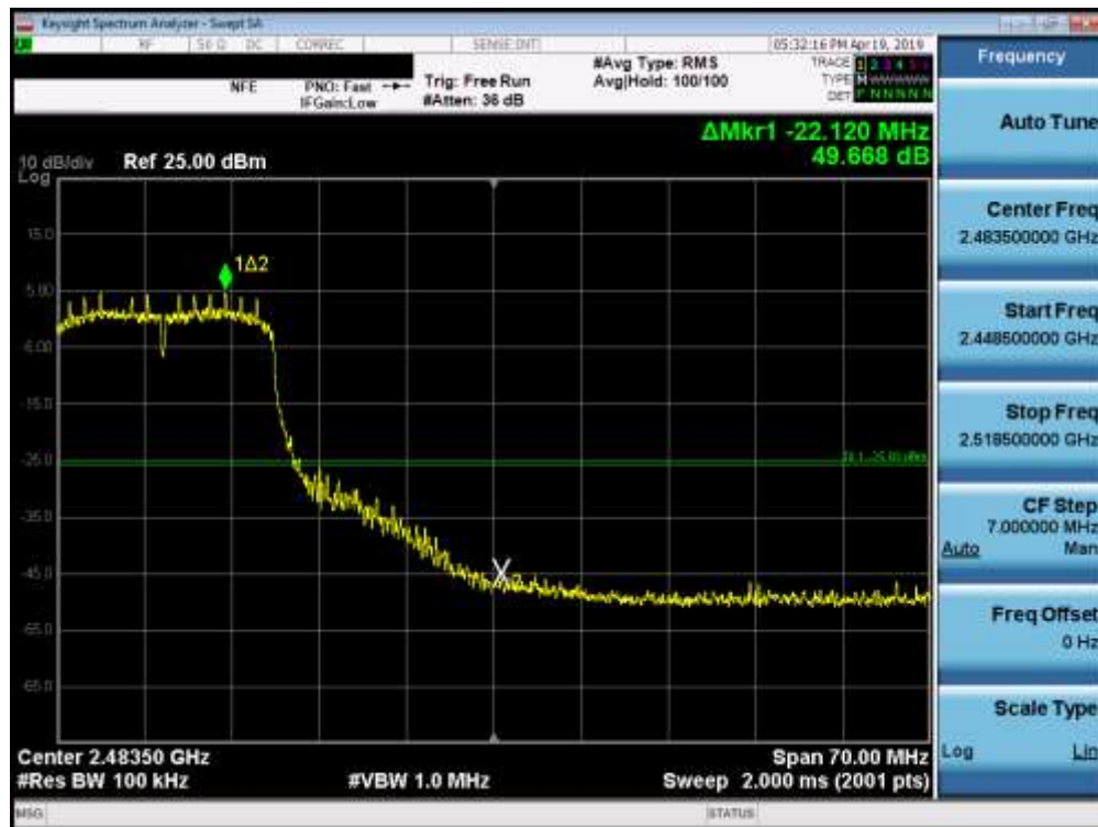
Plot 7-29. Band Edge Plot (802.11n (2.4GHz) – Ch. 10)
