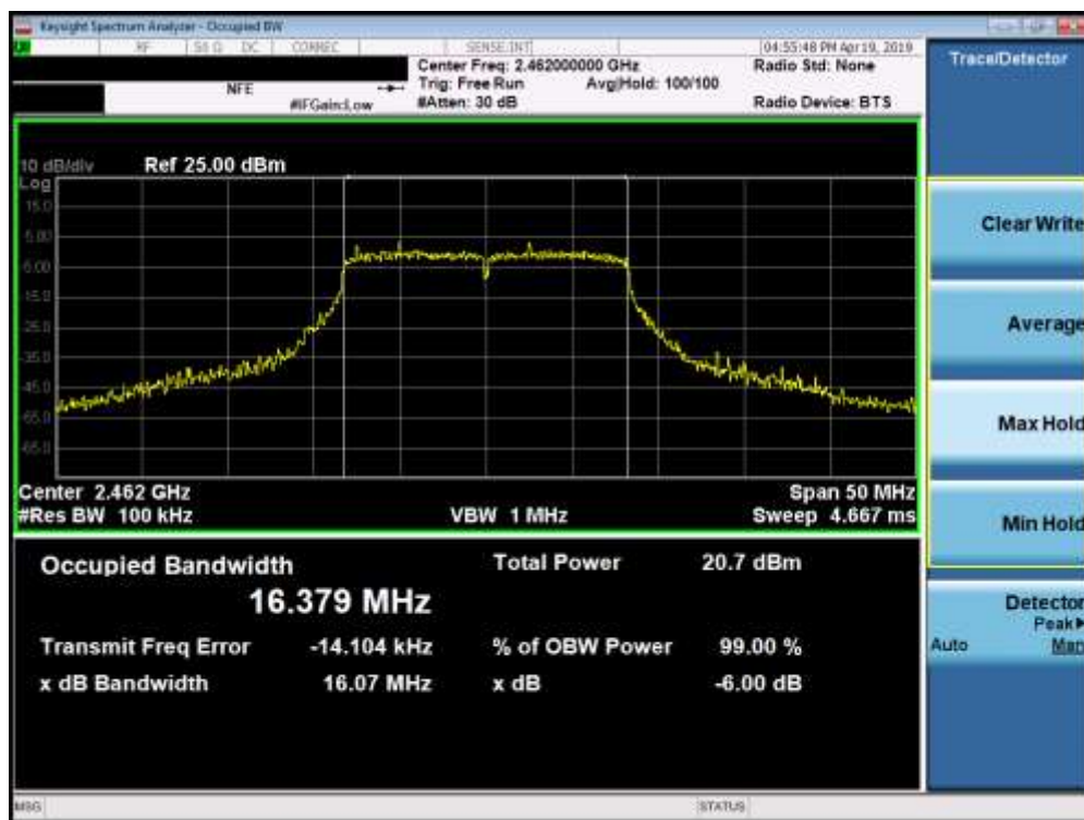
Plot 7-6. 6dB Bandwidth Plot (802.11g – Ch. 11)
