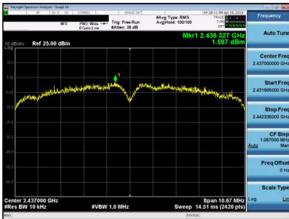
Plot 7-11. Power Spectral Density Plot (802.11b – Ch. 6)
