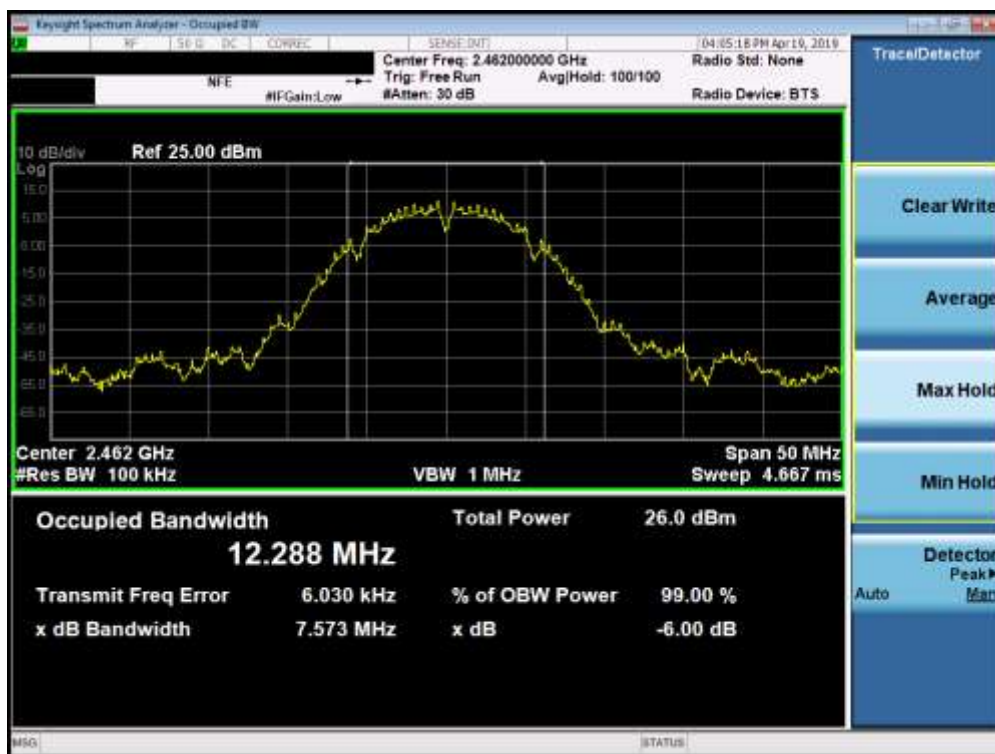
Plot 7-3. 6dB Bandwidth Plot (802.11b – Ch. 11)
