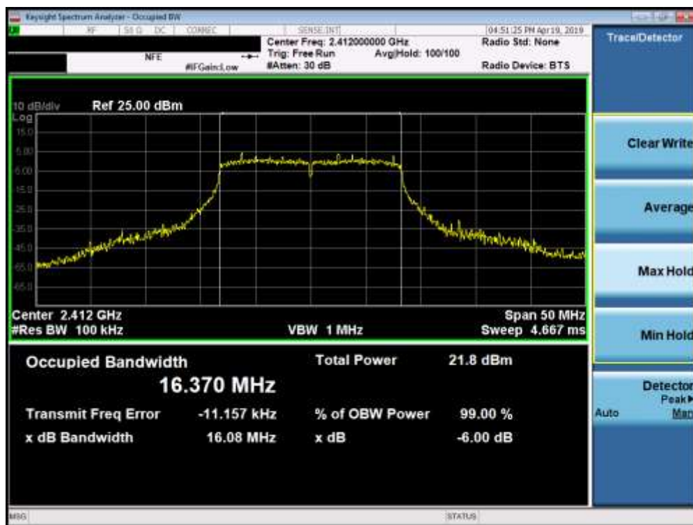
Plot 7-4. 6dB Bandwidth Plot (802.11g – Ch. 1)
