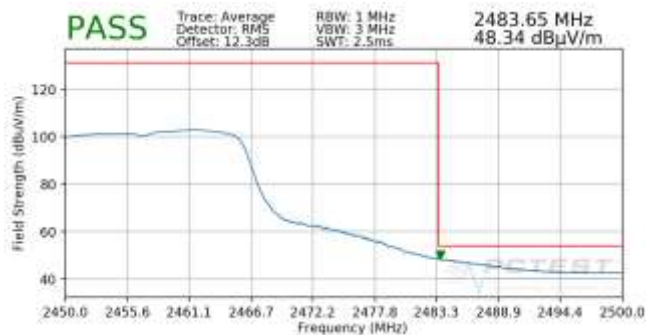
Plot 7-45. Radiated Restricted Upper Band Edge Measurement (Average)
