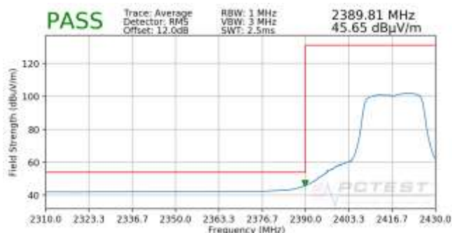
Plot 7-43. Radiated Restricted Lower Band Edge Measurement (Average)
