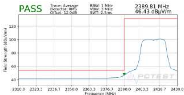
Plot 7-41. Radiated Restricted Lower Band Edge Measurement (Average)
