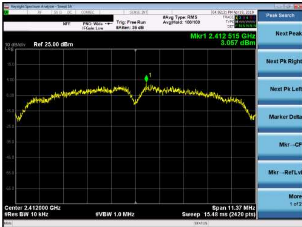
Plot 7-10. Power Spectral Density Plot (802.11b – Ch. 1)
