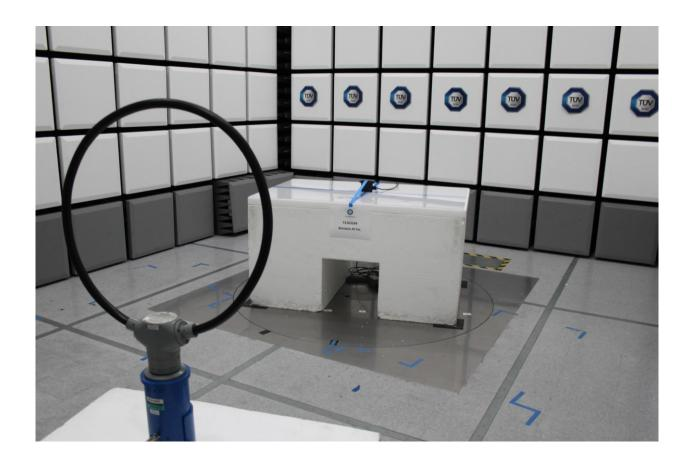
Radiated Emissions Test Setup (Below 30MHz)
