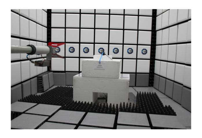
Radiated Emissions Test Setup (1GHz to 18GHz)
