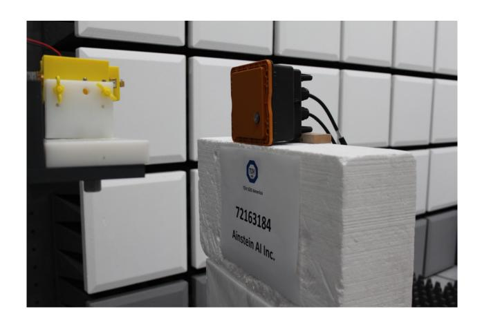
Radiated Emissions Test Setup (Above 18GHz @ 0.2 meter)
