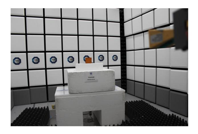
Radiated Emissions Test Setup (Above 18GHz @ 3 meters)
