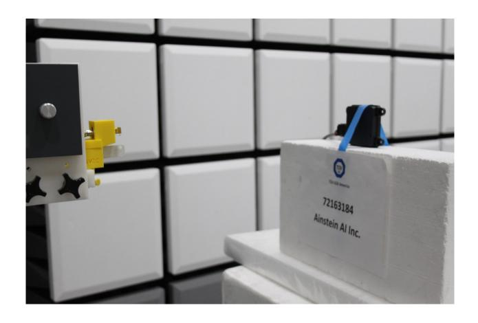
Radiated Emissions Test Setup (Above 18GHz @ 1 meter)
