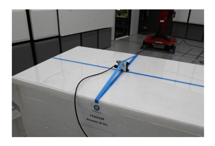
Radiated Emissions Test Setup (30MHz to 1GHz)
