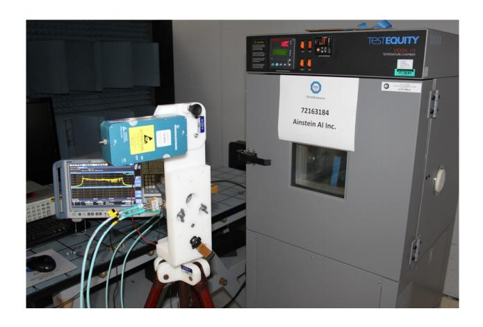
Frequency Stability Test Setup
