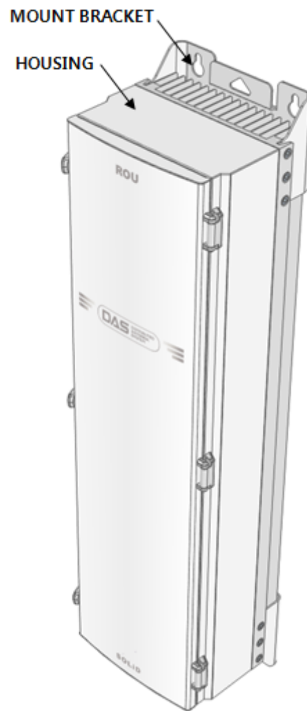
Figure 4.1 – Exterior of Remote Unit
