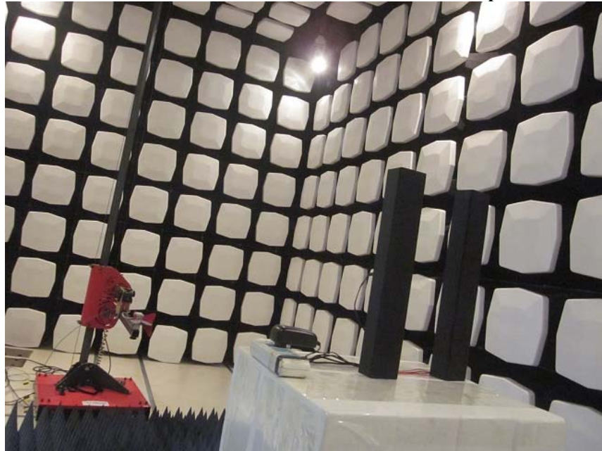
Measurement of Radiated Emission Test Set Up
