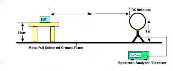
(B) Radiated Emission Test-Up Frequency 30MHz~1GHz
