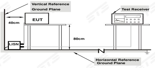
Note: 1.Support units were connected to second LISN.2.Both of LISNs (AMN) are 80 cm from EUT and at least 80 cm from other units and other metal planes support.
