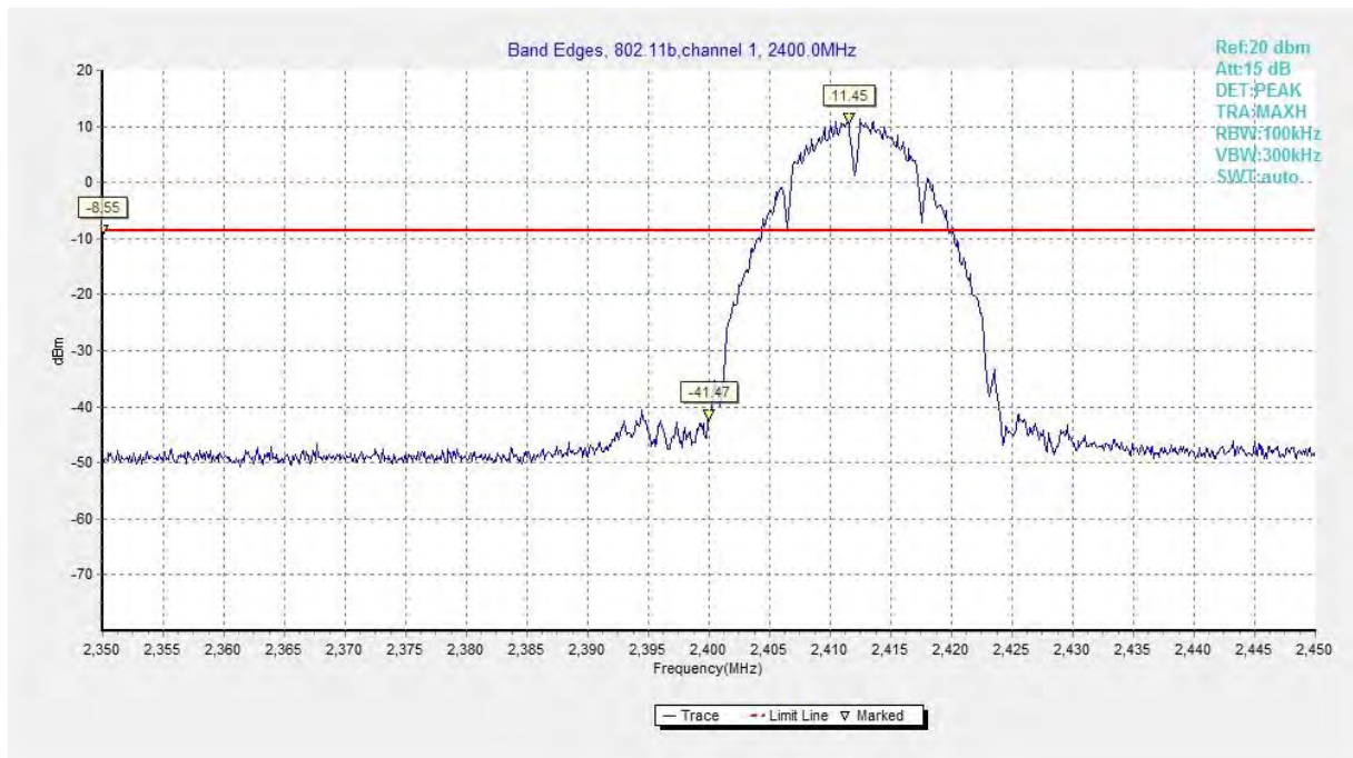
Fig.A.5.1 Band Edges (802.11b, Ch 1)
