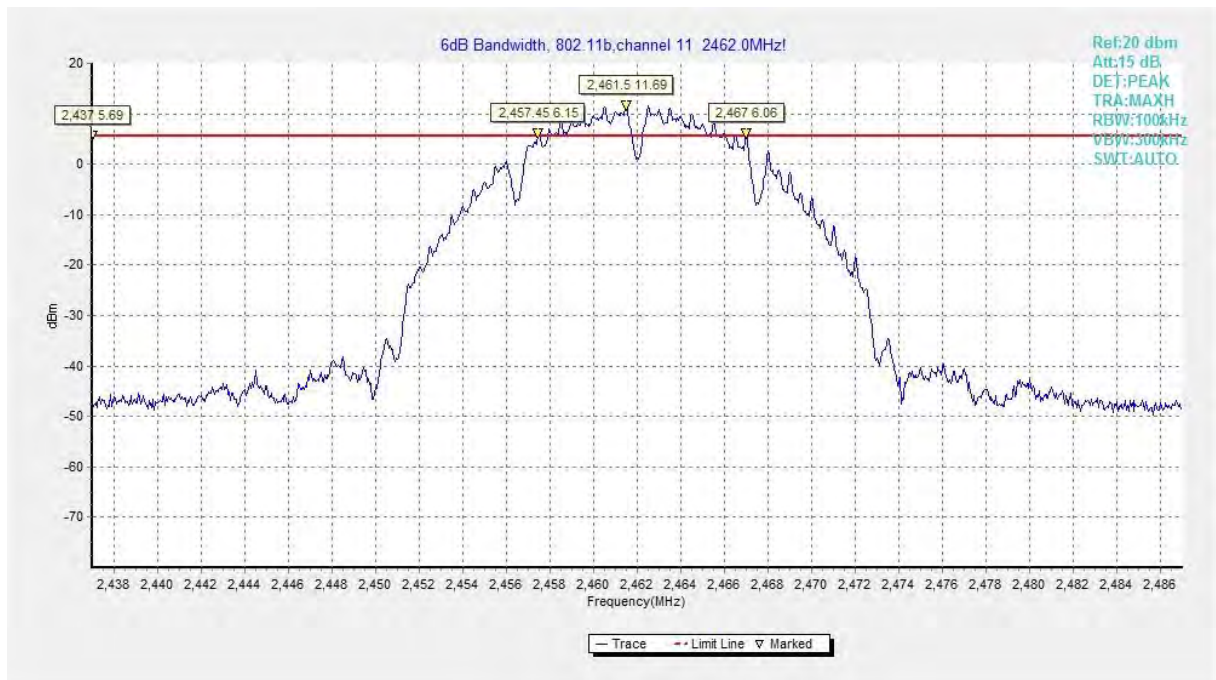
Fig.A.4.3 Occupied 6dB Bandwidth (802.11b, Ch 11)
