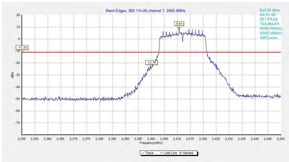
Fig.A.5.5 Band Edges (802.11n-HT20, Ch 1)
