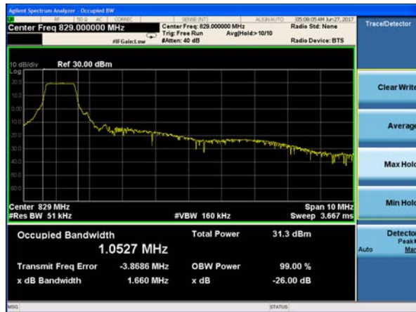
LTE Band 26 16QAM 10MHz CH-Middle
