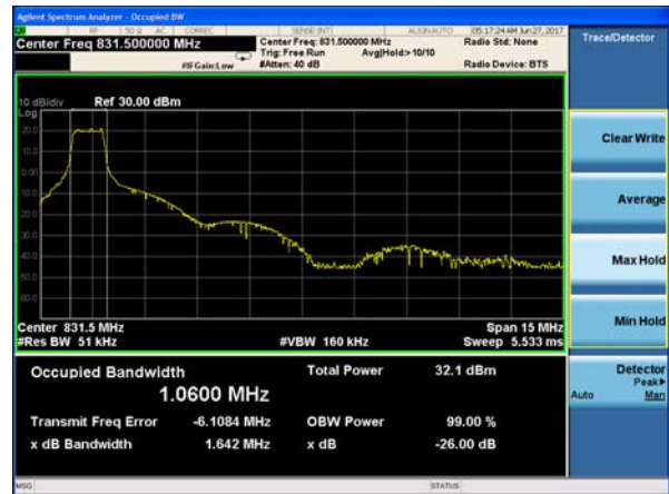
LTE Band 26 16QAM 15MHz CH-Middle
