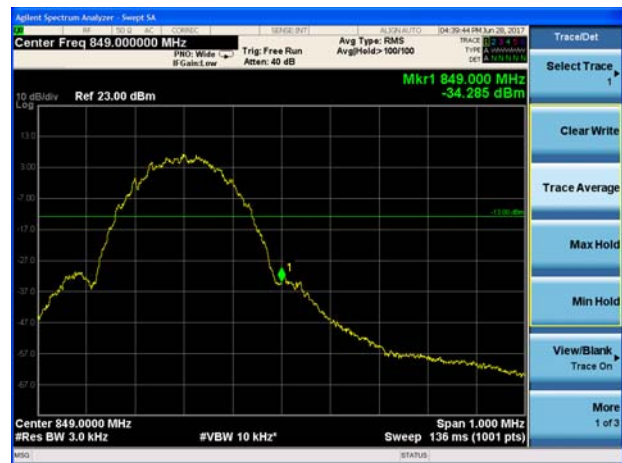
LTE Band 5 QPSK 1.4MHz CH-High 1RB
