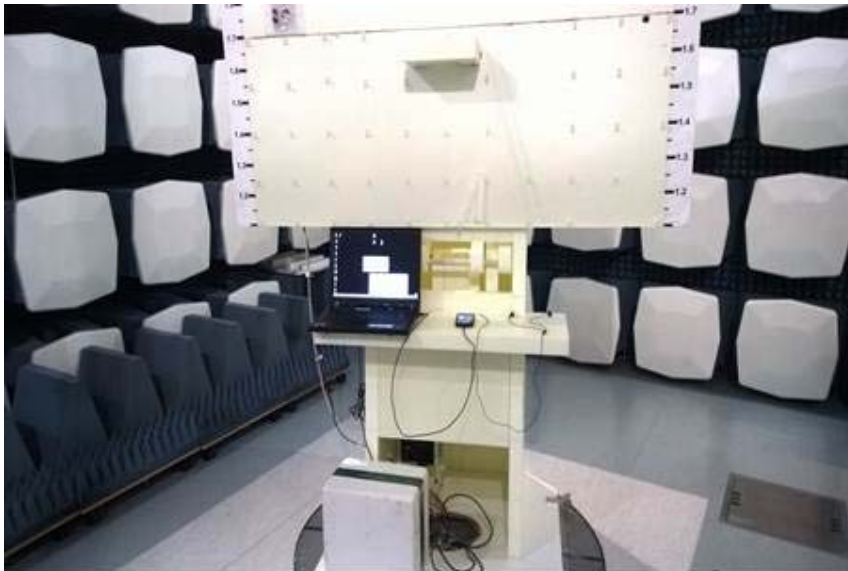
Picture 2. FCC Part 15B Radiated emissions
