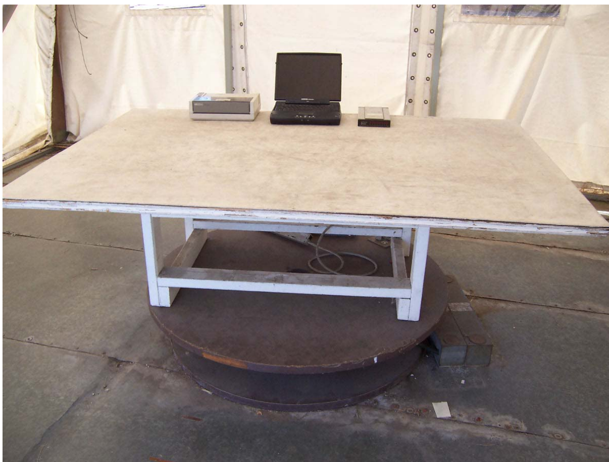
Radiated Emissions Test Setup
