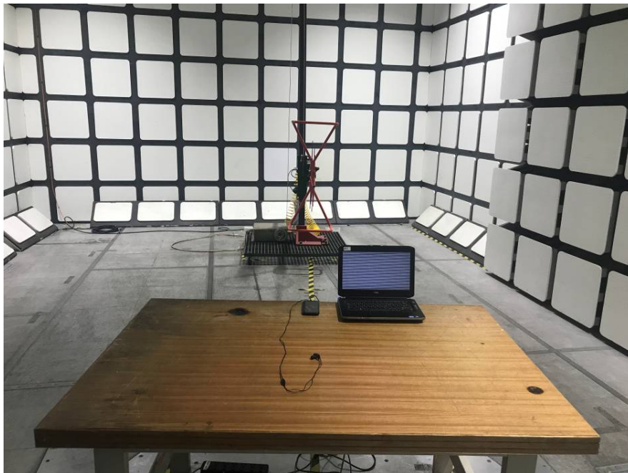
Radiated Emissions – Front View (Below 1 GHz)
