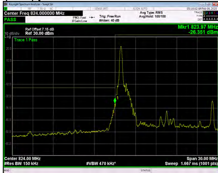
Band26(824-849) QPSK BW=15MHz Channel=26865 RB Size=1 Position=#Max Extended
