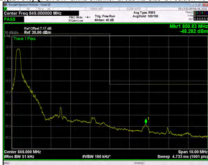
Band26(824-849) QPSK BW=5MHz Channel=27015 RB Size=1 Position=#Max Extended
