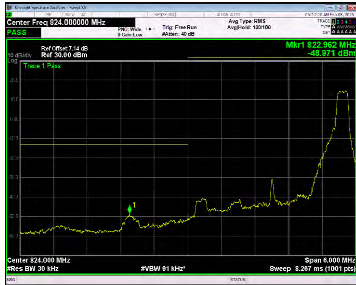
Band26(824-849) 16QAM BW=3MHz Channel=26805 RB Size=15 Position=#0 Extended
