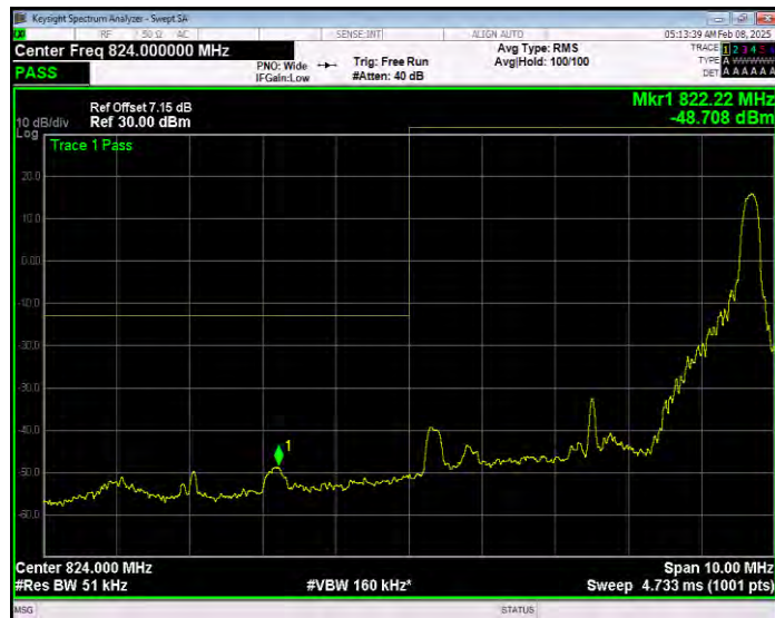
Band26(824-849) 16QAM BW=5MHz Channel=26815 RB Size=25 Position=#0 Extended
