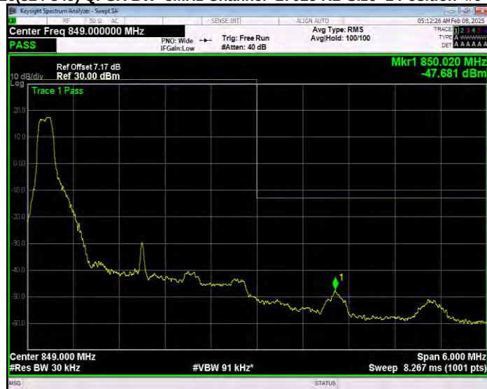
Band26(824-849) QPSK BW=3MHz Channel=27025 RB Size=1 Position=#Max Extended
