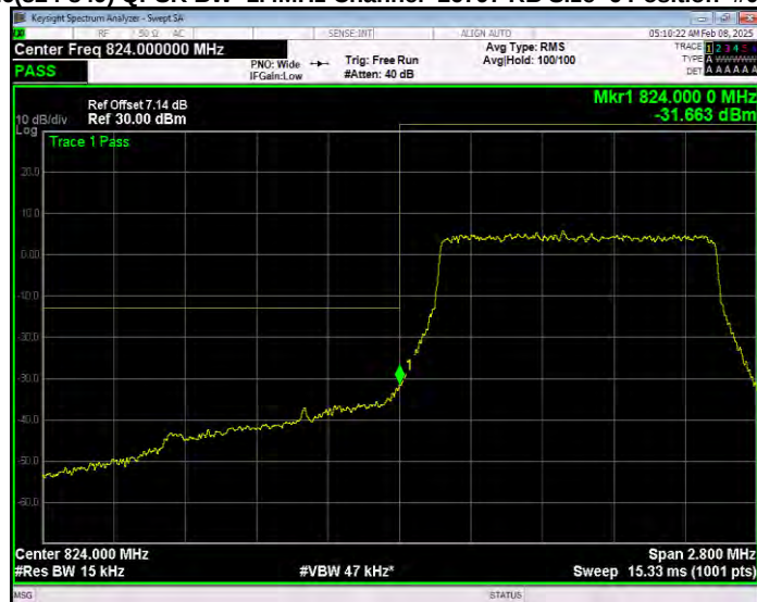
Band26(824-849) QPSK BW=1.4MHz Channel=27033 RB Size=1 Position=#0 Extended
