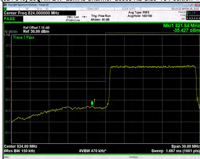
Band26(824-849) 16QAM BW=15MHz Channel=26965 RB Size=1 Position=#0 Extended
