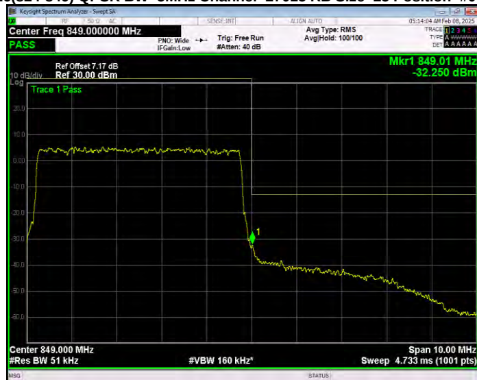
Band38 16QAM BW=10MHz Channel=37800 RB Size=1 Position=#0 Extended
