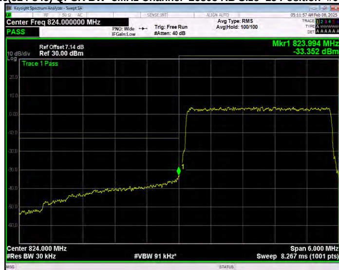
Band26(824-849) QPSK BW=3MHz Channel=27025 RB Size=1 Position=#0 Extended
