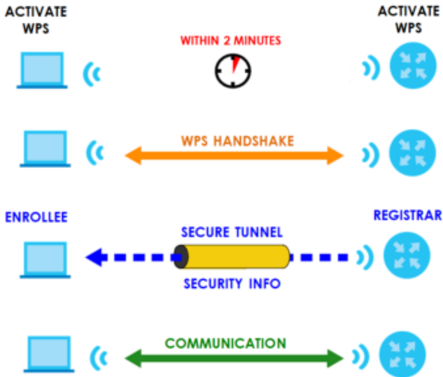
Figure 69 How WPS Works
