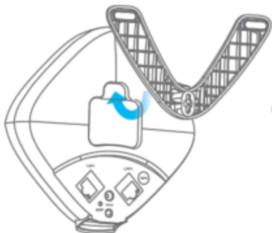
Figure 20 Attach the bracket
