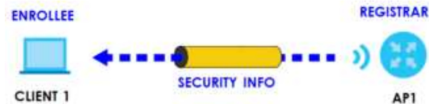
Figure 70 WPS: Example Network Step 1
