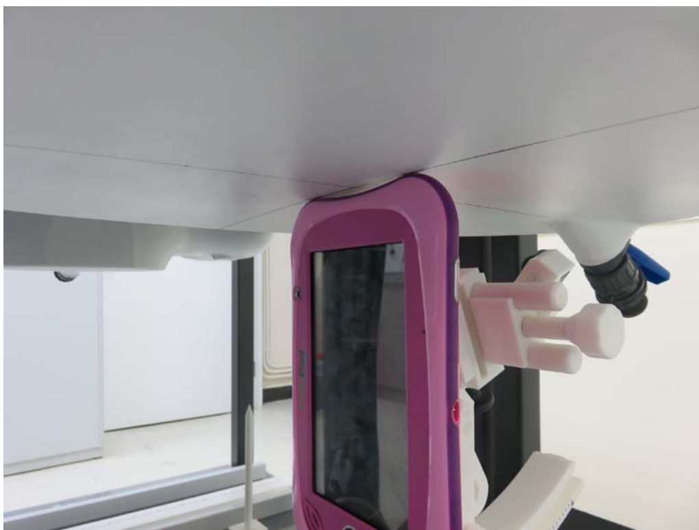
Figure 4 – Right surface with 0mm Separation
