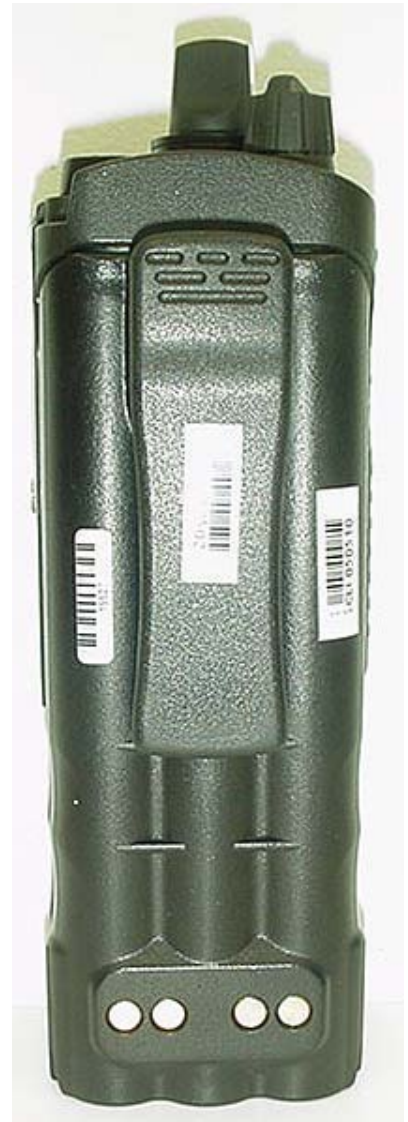
Back of DUT with NiMH Battery Pack with Belt-Clip
