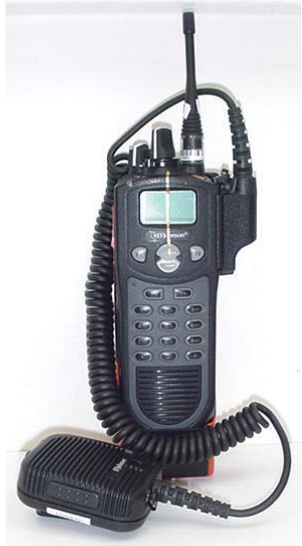
Radio with Speaker-Microphone Accessory & Alkaline Battery Pack
