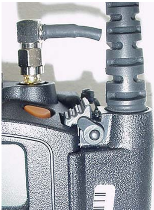
Front View of Antenna Termination
