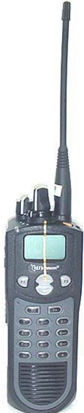
Front of DUT with Whip Antenna & NiMH Battery Pack
