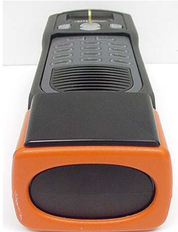
Bottom of DUT with Alkaline Battery Pack
