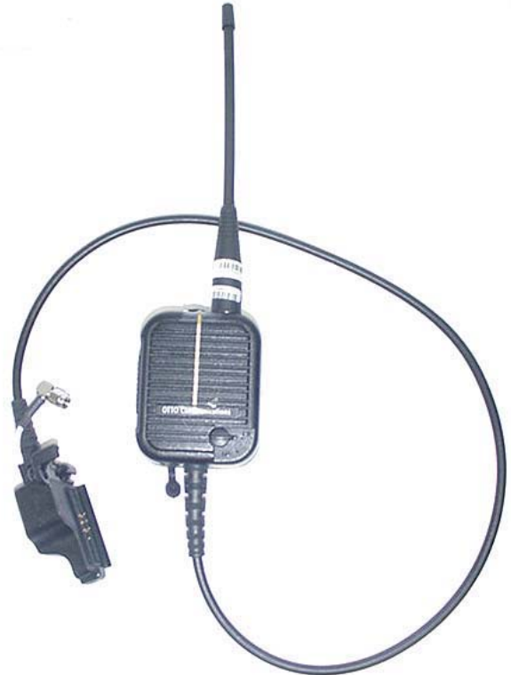
Speaker-Microphone with Whip Antenna
