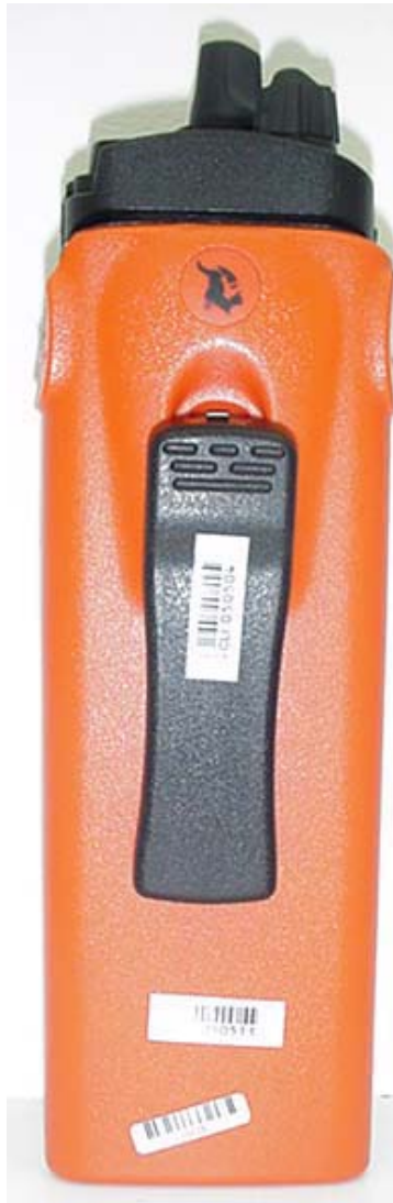
Back of DUT with Alkaline Battery Pack & Belt-Clip
