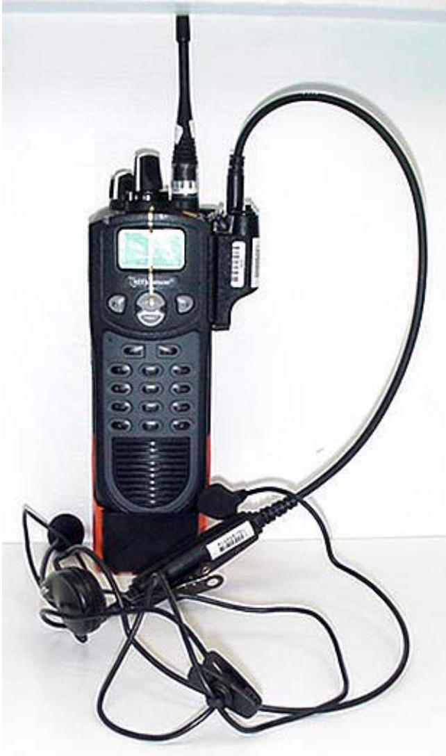
Radio with Boom-Microphone Headset Accessory & Alkaline Battery Pack
