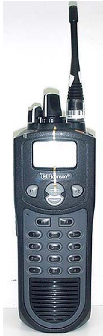
Front of DUT with Stubby Antenna & NiMH Battery Pack
