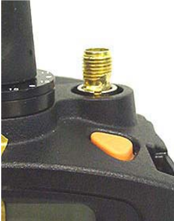
Radio RF Antenna Connector
