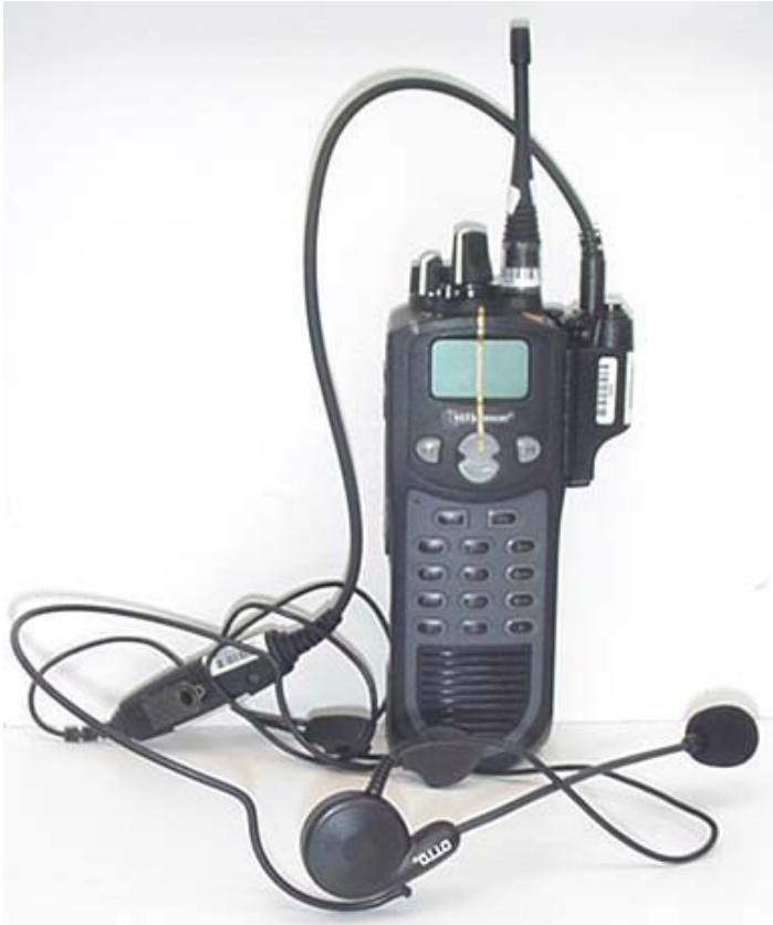
Radio with Boom-Microphone Headset Accessory & NiMH Battery Pack
