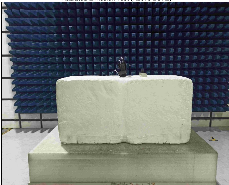
Radiated Emission Test (Above 1GHz)
