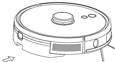
Press and hold the button in the middle of the tank and push it horizontally along the rear of the robot. The module is intalled in place if you hear the sound of "click".
