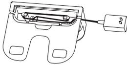
2. Place charging base against the wall and connect the power.
