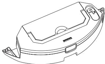
Please put the dustbin into the water tank and put the handle in the slot.
