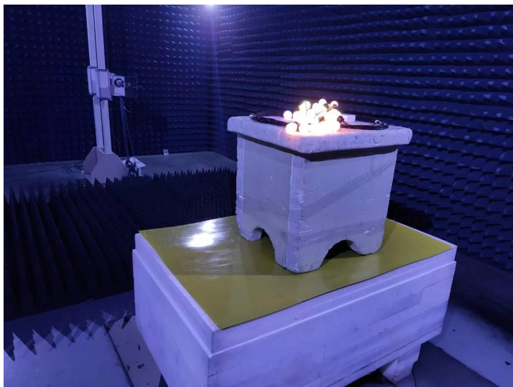
Photo of Radiated Emission Measurement (Above 1G)
