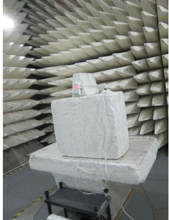
EUT powered via adapter
