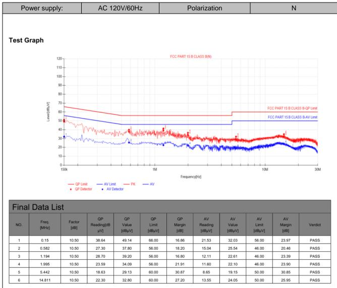
Note:1).QP Value (dBµV)= QP Reading (dBµV)+ Factor (dB)
