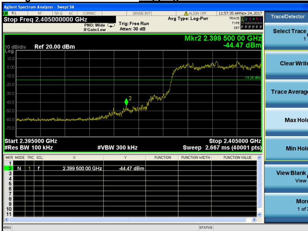
Conducted Spurious Emissions *Lowest Channel & Modulation : 8DPSK*
