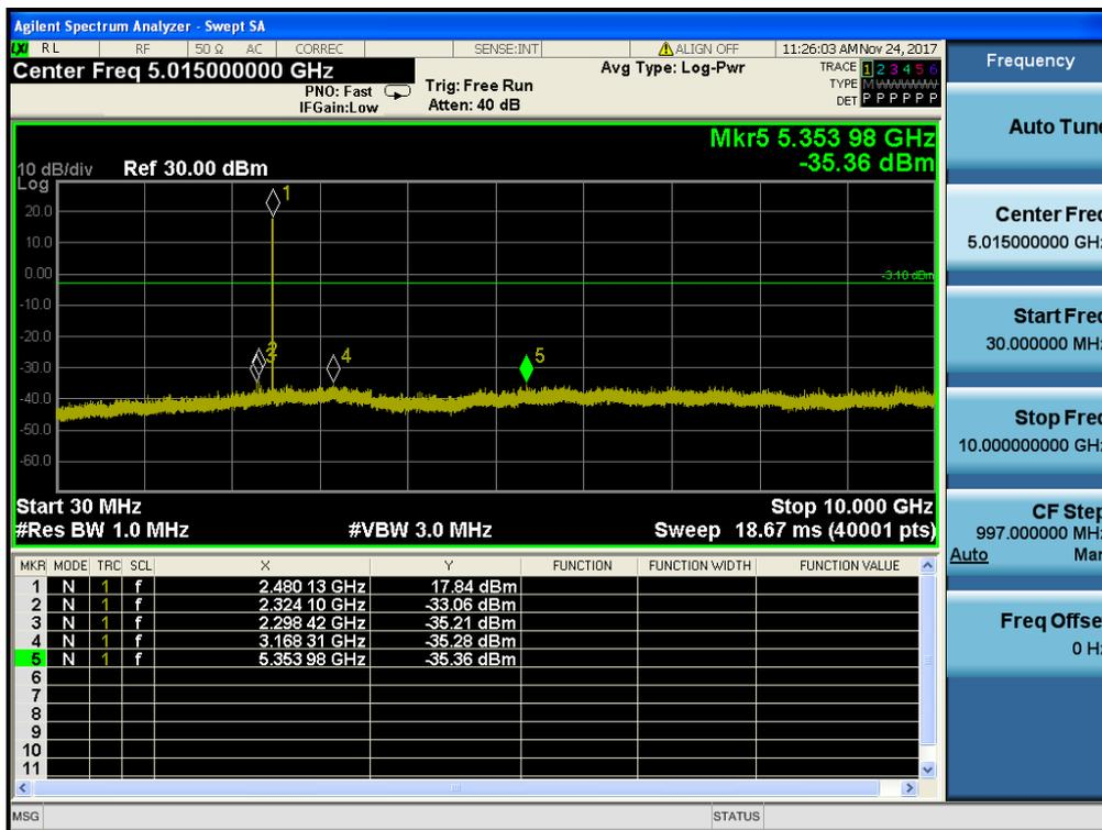
Conducted Spurious Emissions *Highest Channel & Modulation : GFSK*
