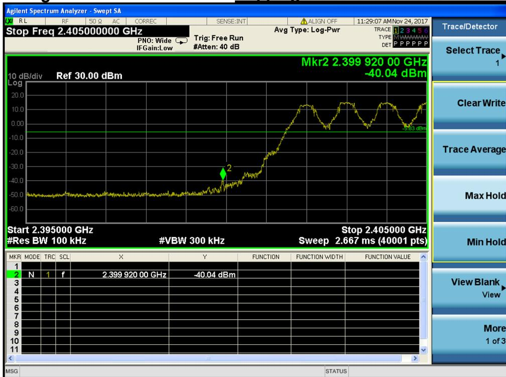
Conducted Spurious Emissions *Lowest Channel & Modulation : GFSK*
