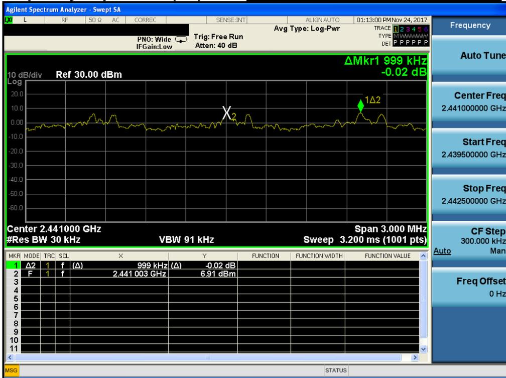
**Carrier Frequency Separation (AFH) *Hopping mode : Enable & GFSK***
