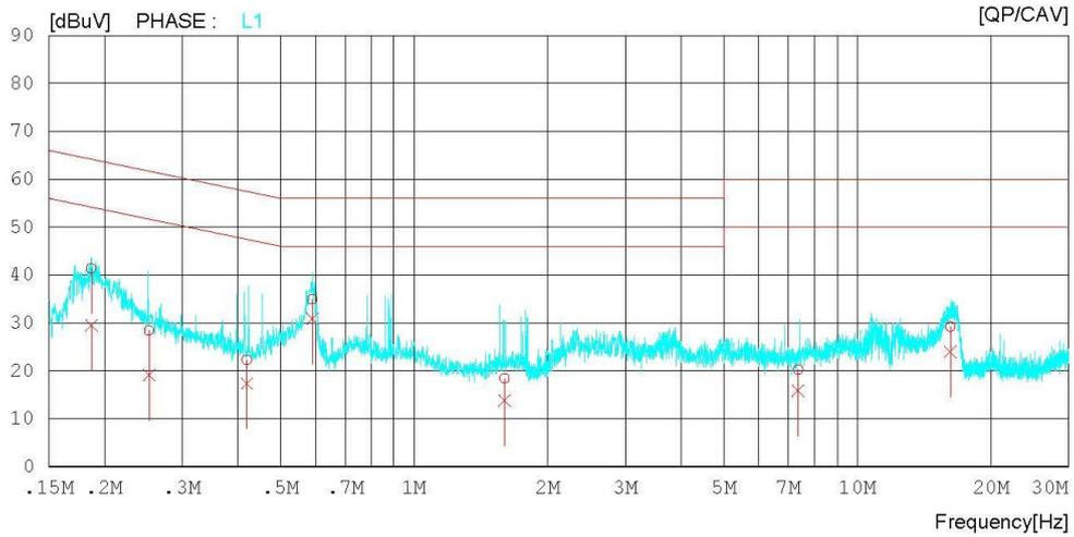
**AC Line Conducted Emissions (List) = Modulation : GFSK**
