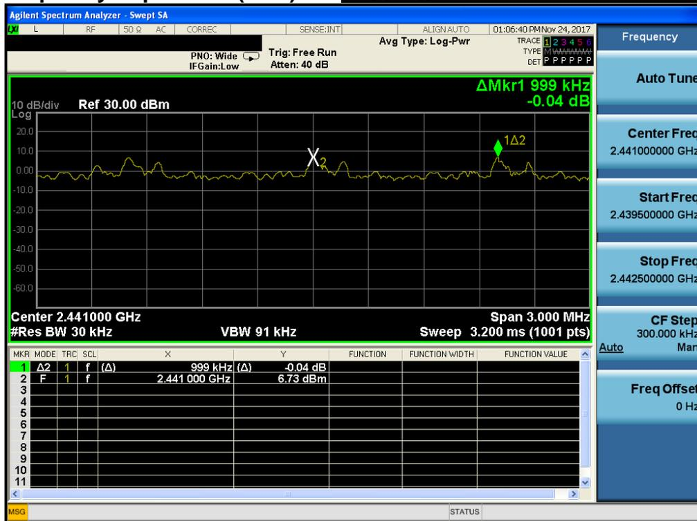
Carrier Frequency Separation (AFH) *Hopping mode : Enable & 8DPSK*
