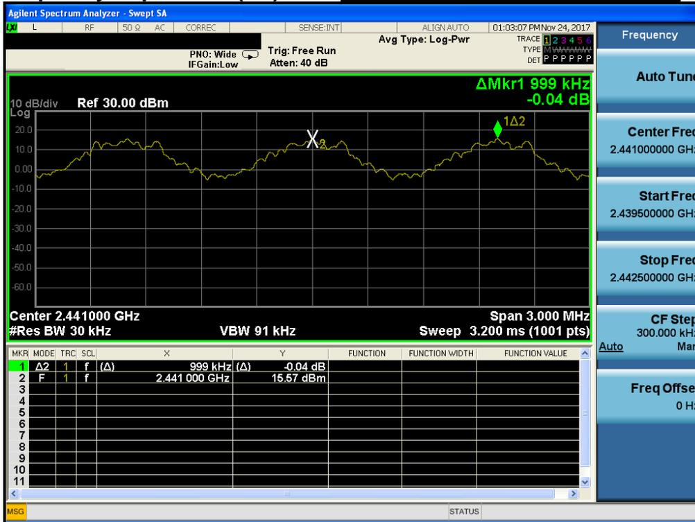
**Carrier Frequency Separation (FH) *Hopping mode : Enable & π/4-DQPSK***
