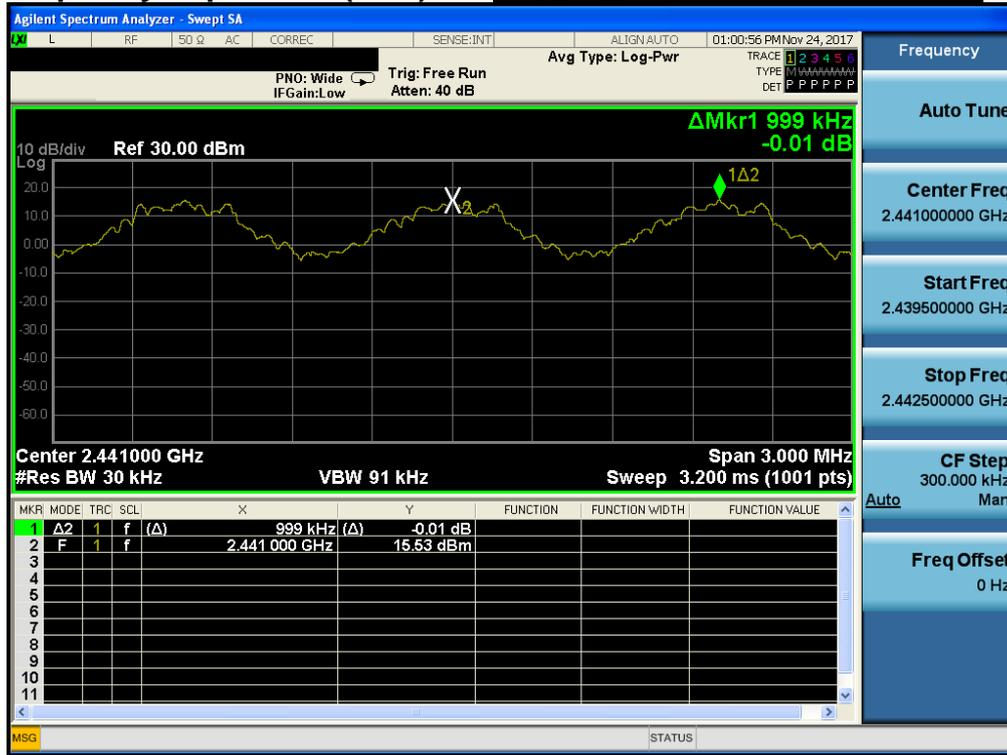
**Carrier Frequency Separation (AFH) *Hopping mode : Enable & π/4-DQPSK***
