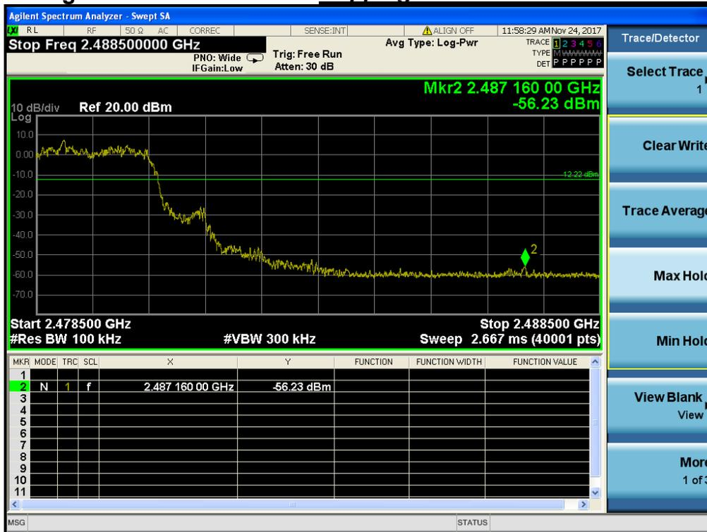
Conducted Spurious Emissions **Highest Channel & Modulation : 8DPSK**
