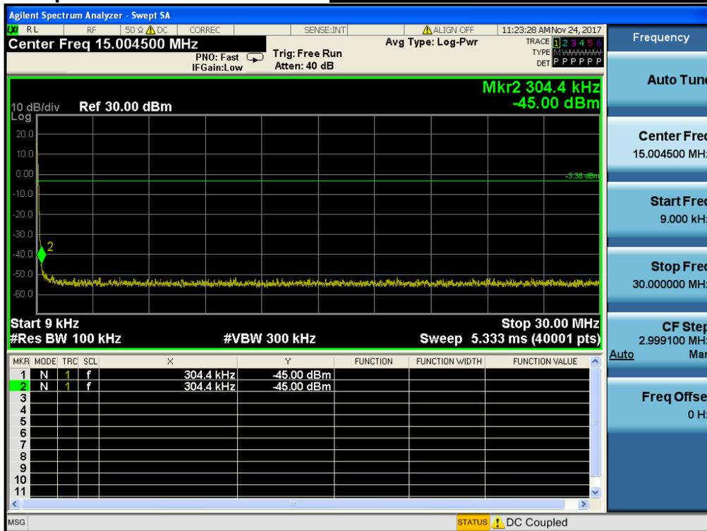
Conducted Spurious Emissions *Middle Channel & Modulation : GFSK*
