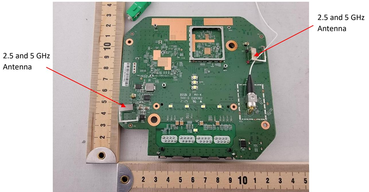
**Photograph 4: Top View of Circuit Board**
