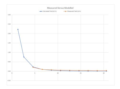
Calculated field based on the following (source: Magnetic Field of a Current Loop (gsu.edu))
