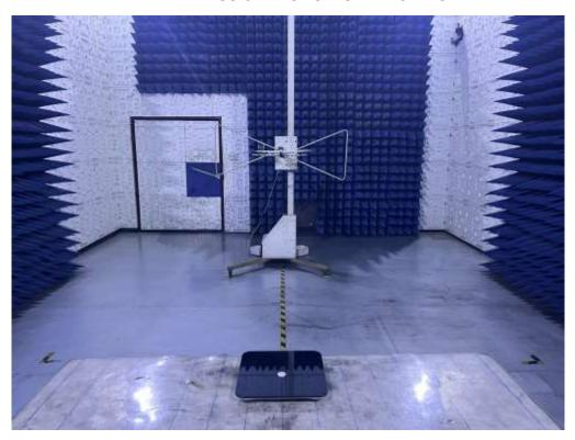
RADIATED EMISSION TEST SETUP ABOVE 1GHz
