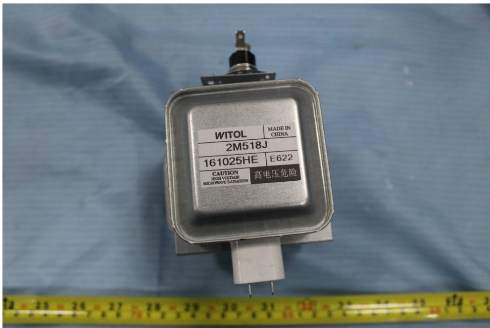
EUT – Magnetron Label View
