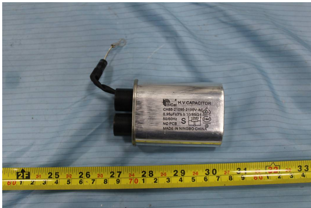
EUT – High Voltage Capacitor View
