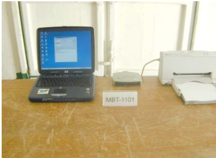
Photo 2: Radiated Spurious Test Set-up (rear)
