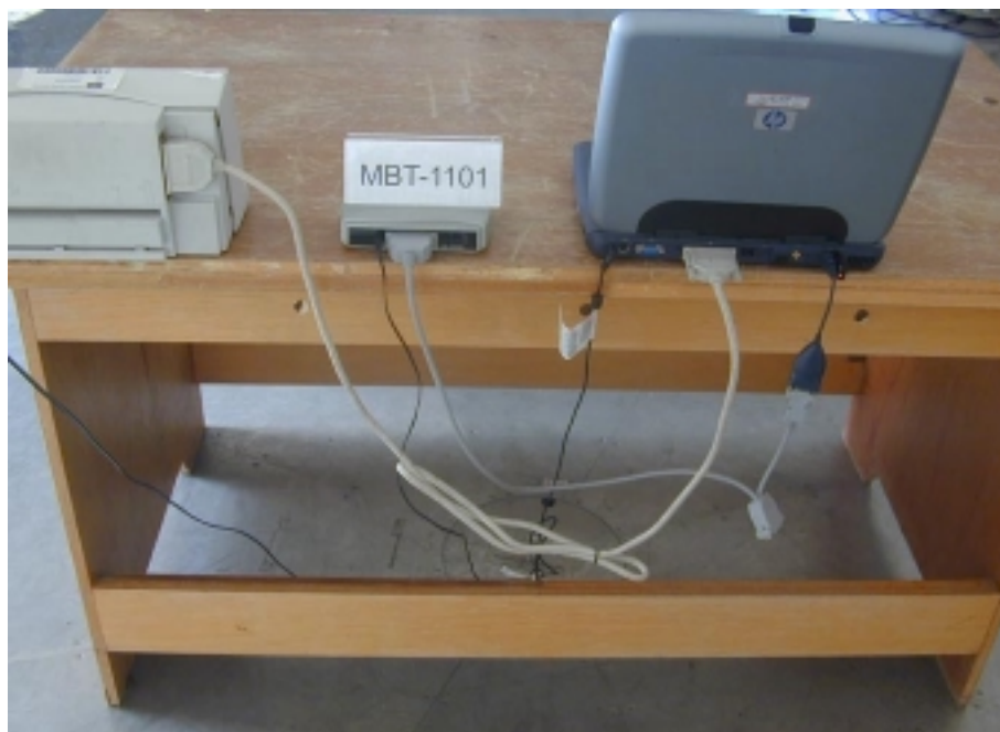
Photo 2: Radiated Spurious Test Set-up (rear)
