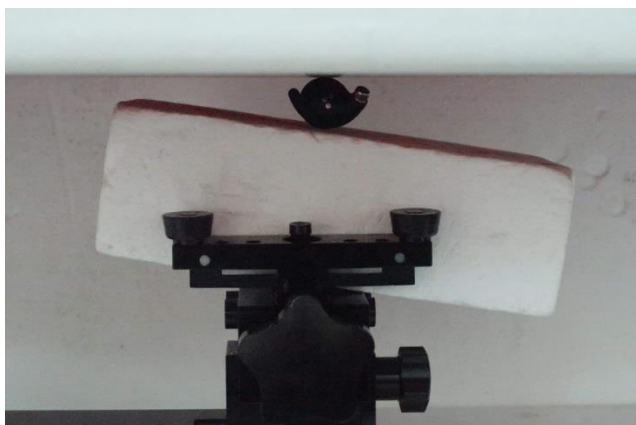
Antenna Side, Test Separation 0 mm
