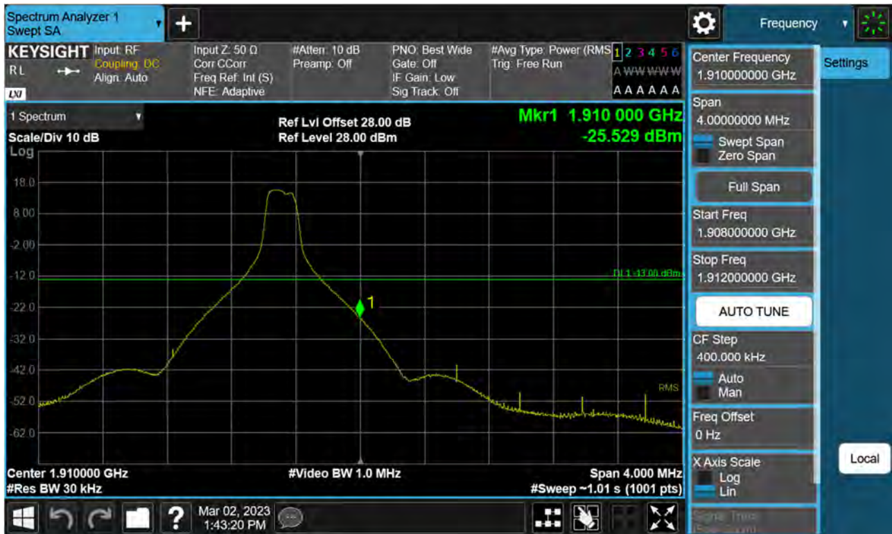
Sub6 n2. Upper Band Edge Plot (15 M BW Ch.380500 BPSK_RB1_Offset 78) -1
