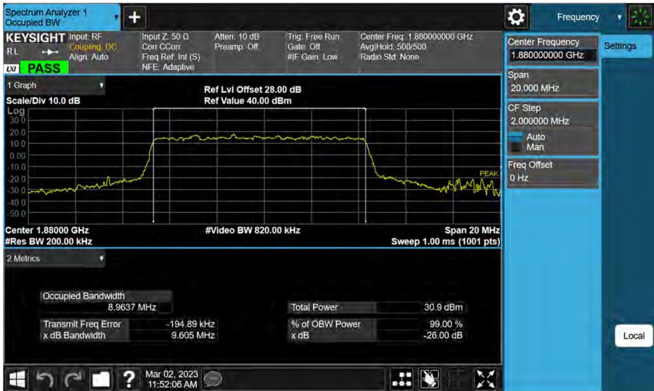
Sub6 n2. Occupied Bandwidth Plot (10 M BW Ch.376000 QPSK RB 50_0)
