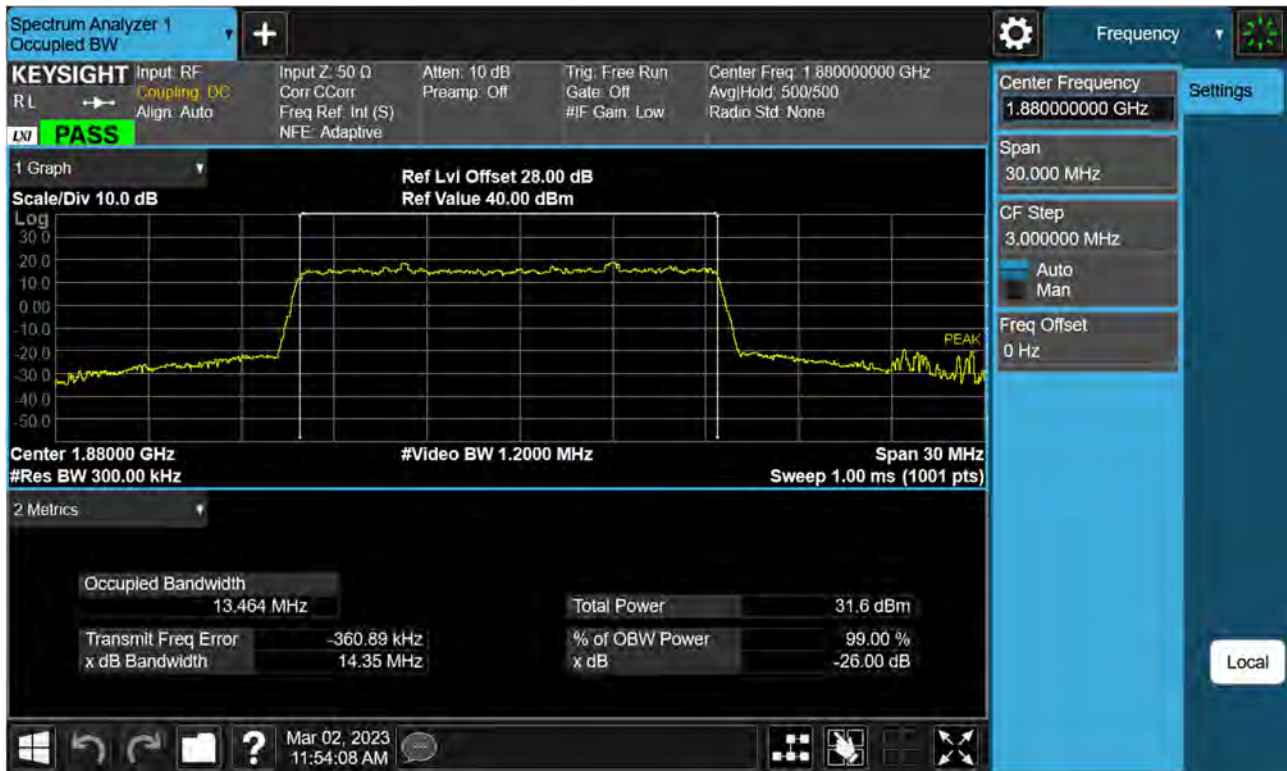
Sub6 n2. Occupied Bandwidth Plot (15 M BW Ch.376000 BPSK RB 75_0)
