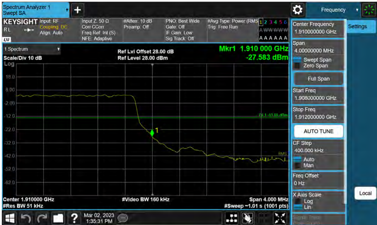
Sub6 n2. Upper Band Edge Plot (5 M BW Ch.381500 BPSK_RB25_Offset 0) -2
