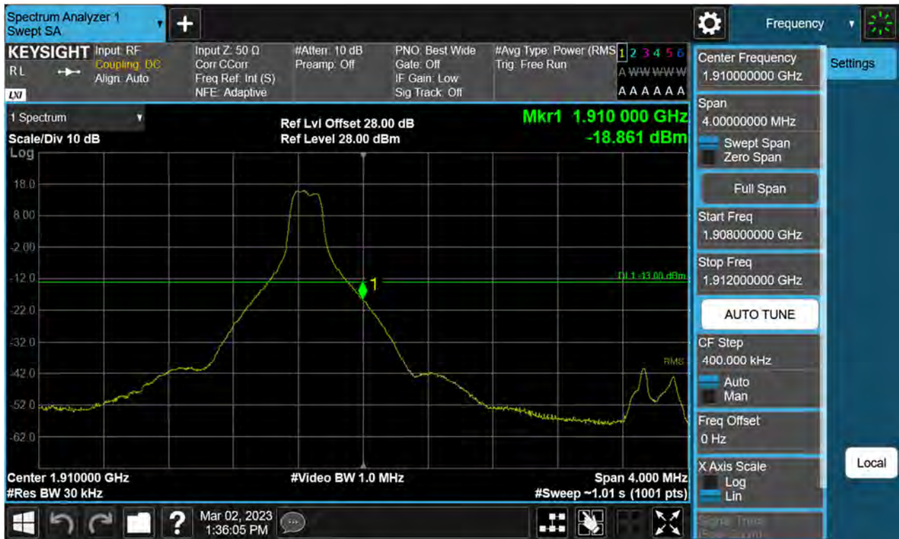
Sub6 n2. Upper Band Edge Plot (5 M BW Ch.381500 BPSK_RB1_Offset 24) -1
