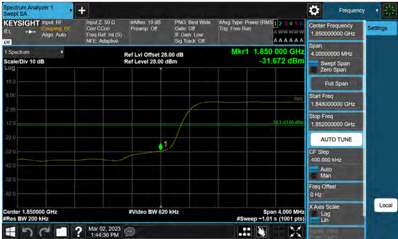
Sub6 n2. Lower Band Edge Plot (20 M BW Ch.372000 BPSK_RB100_Offset 0) -2
