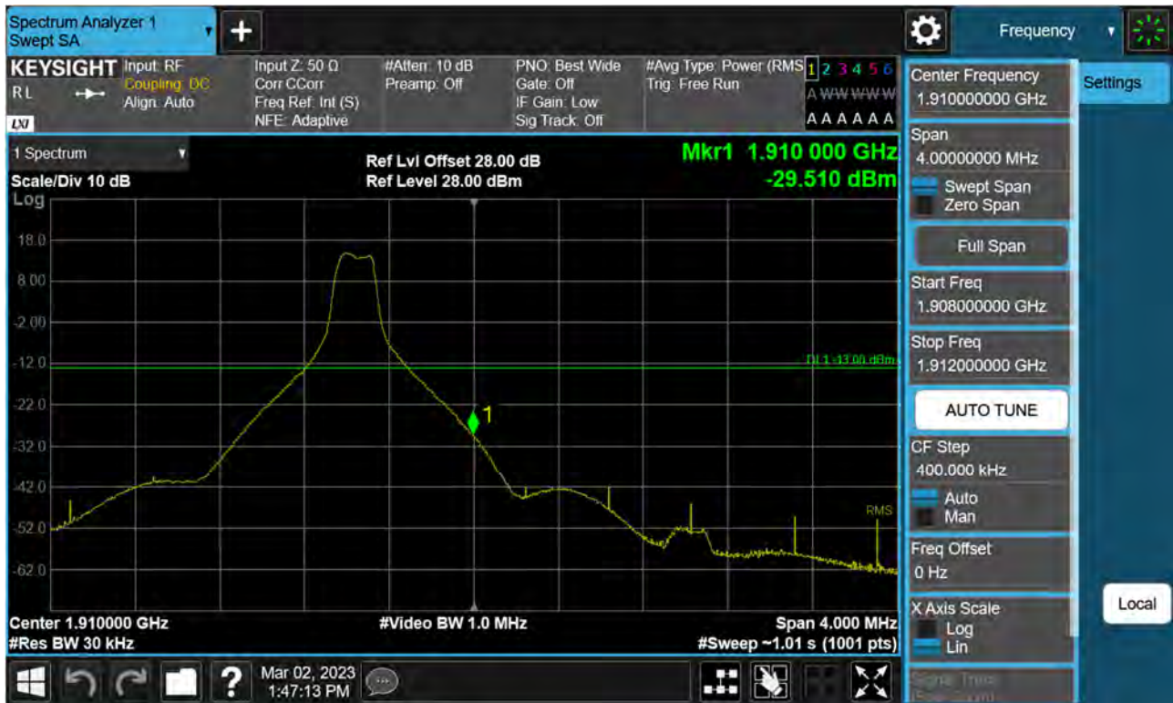
Sub6 n2. Upper Band Edge Plot (20 M BW Ch.380000 BPSK_RB1_Offset 105) -1
