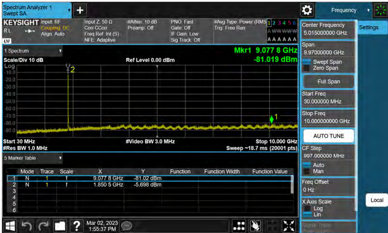
Sub6 n2. Conducted Spurious_1 (371000ch_10 MHz_BPSK_RB 1_1)
