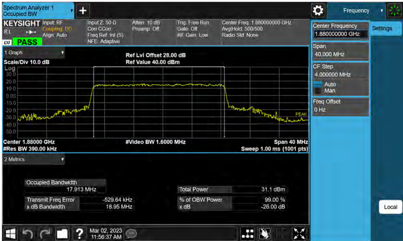
Sub6 n2. Occupied Bandwidth Plot (20 M BW Ch.376000 QPSK RB 100_0)
