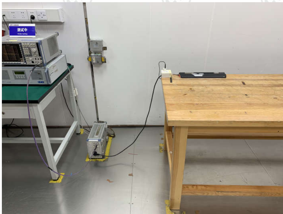
Conducted Emissions Test Setup
