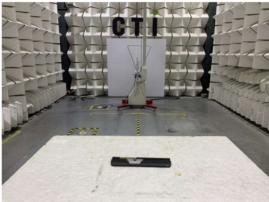
Radiated spurious emission Test Setup-1(Below 1GHz)
