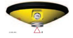
a The Antenna Reference Plane is the underside of the threaded metal insert.
