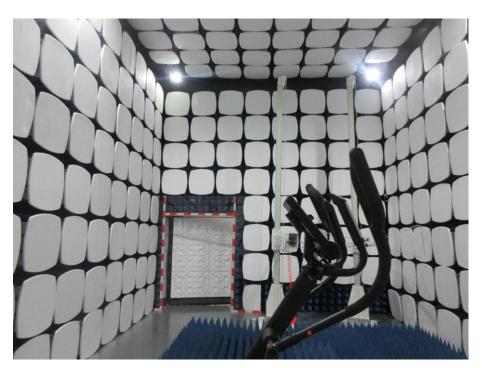
Remark: The transmitter part of the EUT was kept on the high 1.5m above 1GHz according to the lifting platform during the test.
