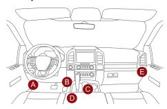
Usually, the OBD port is located under the dashboard, above the pedal on the driver's side. The five locations shown in the picture are common OBDII port locations.
