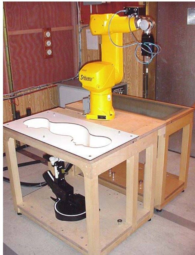
DASY4 SAR Measurement System with SAM validation phantom
