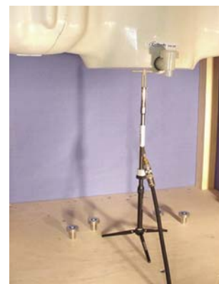
1800MHz Dipole Setup
