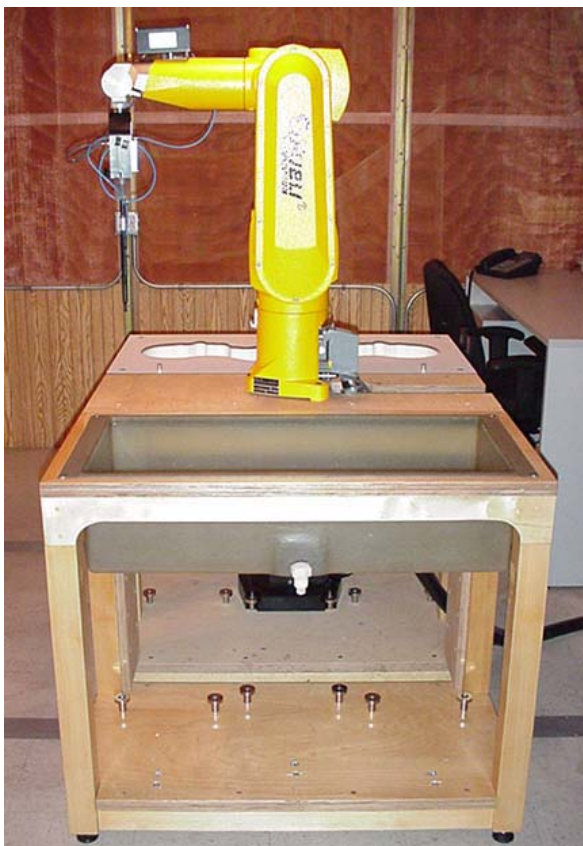
DASY4 SAR Measurement System with planar phantom
