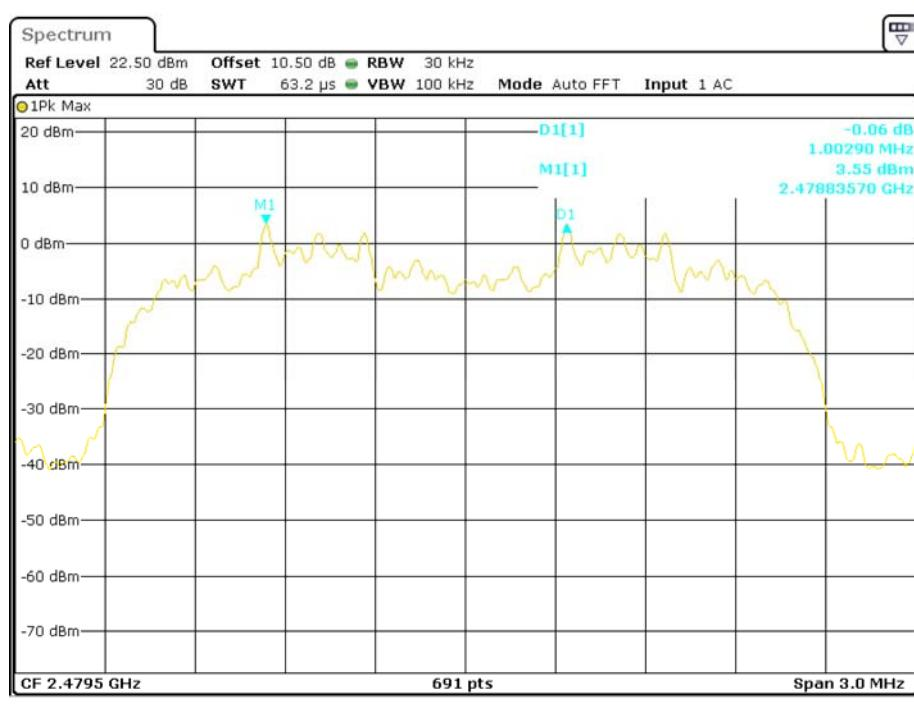
**EDR (8DPSK): Low Channel**
