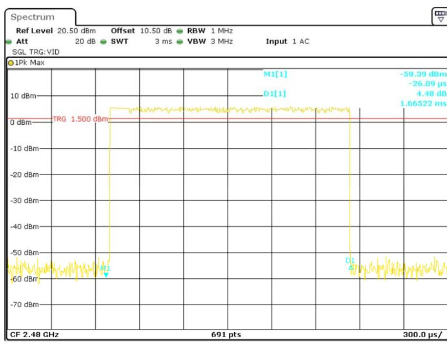
**Pulse time, Low Channel, 3DH5**
