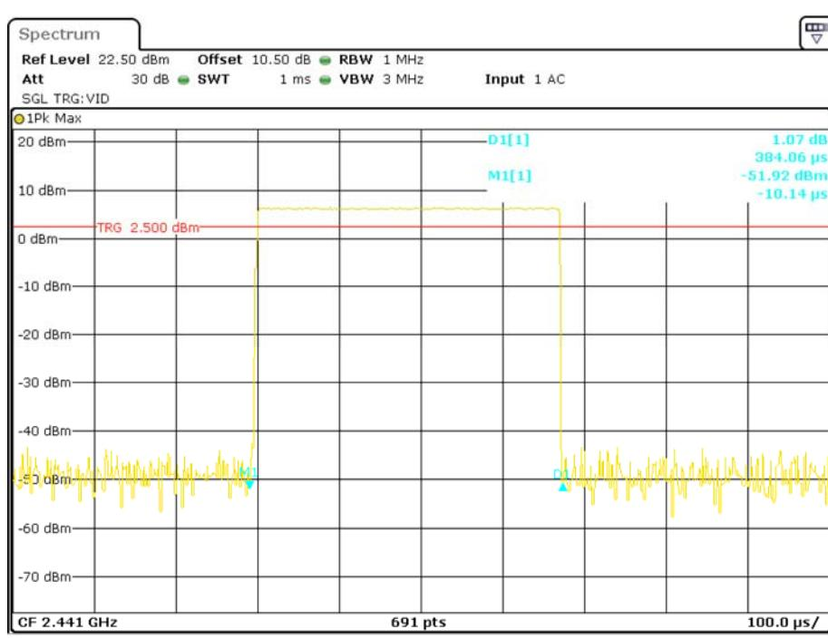
**Pulse time, High Channel, DH1**
