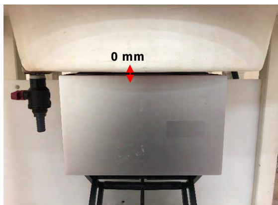
Fig.3 EUT Bottom side to flat phantom
