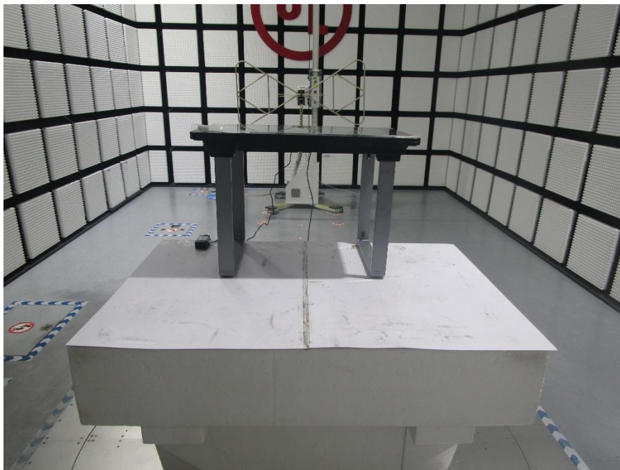
RADIATED RF MEASUREMENT SETUP (30MHz~1GHz)
