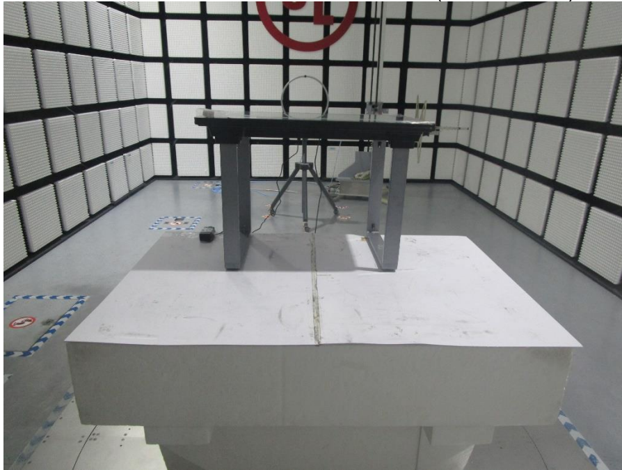
RADIATED RF MEASUREMENT SETUP (Below 30MHz)
