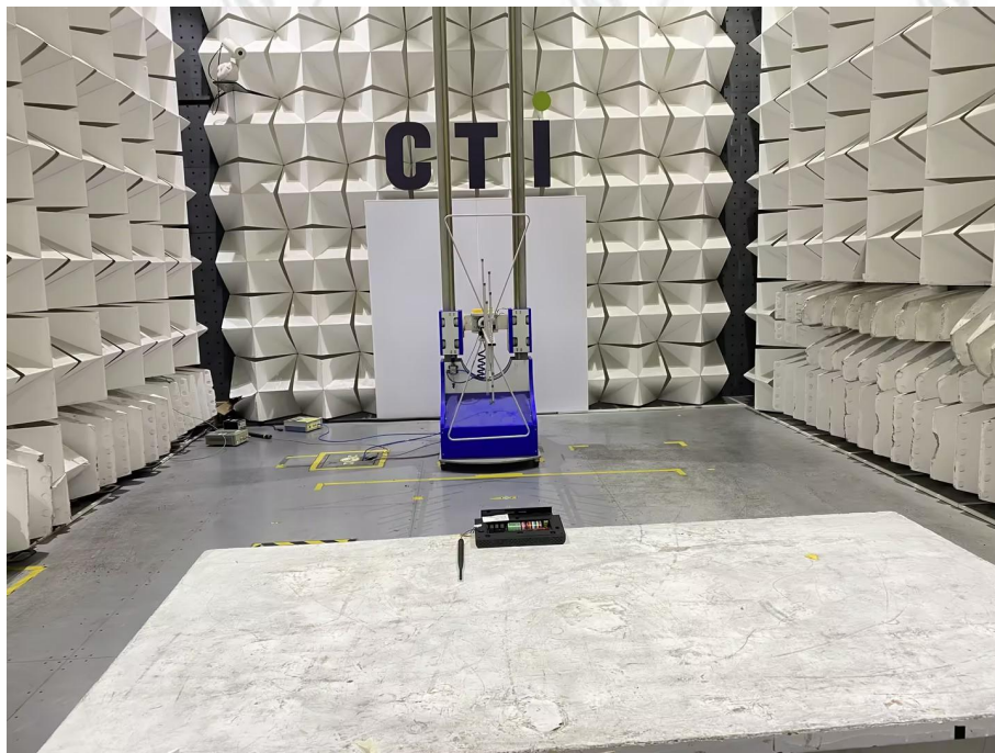
Radiated spurious emission Test Setup-1(Below 1GHz)
