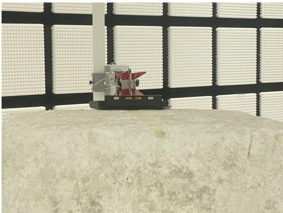
Radiated spurious emission Test Setup-2(Above 1GHz)
