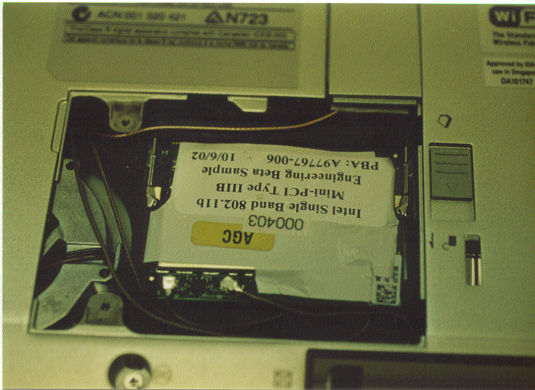
View Transmitter Inside the Portege Laptop
