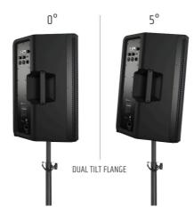
The speakers are equipped with a stand adapter with a stand connection with an angle of 0° (rear position) and a stand connection with a tilt angle of 5° (front position). Examples of use: Use the stand adapter with an angle of 0° for emitting sound to a public audience and the stand adapter with a tilt angle of 5° for emitting sound to a seated audience.
