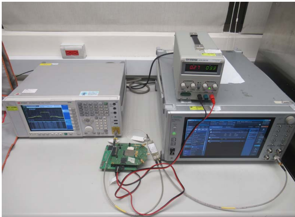
Conducted Setup Photo (Measurement at Antenna Port)
