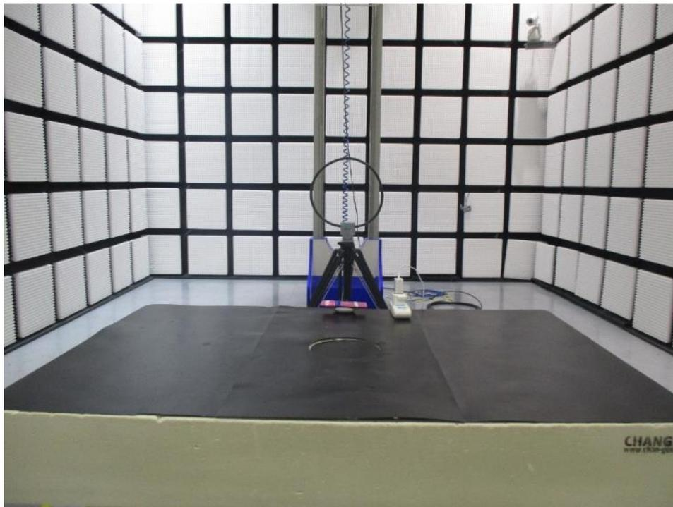
Radiated Disturbance Emissions (9kHz-30MHz)
