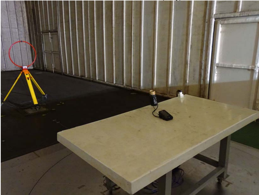
Front View of Radiated Test (Loop)
