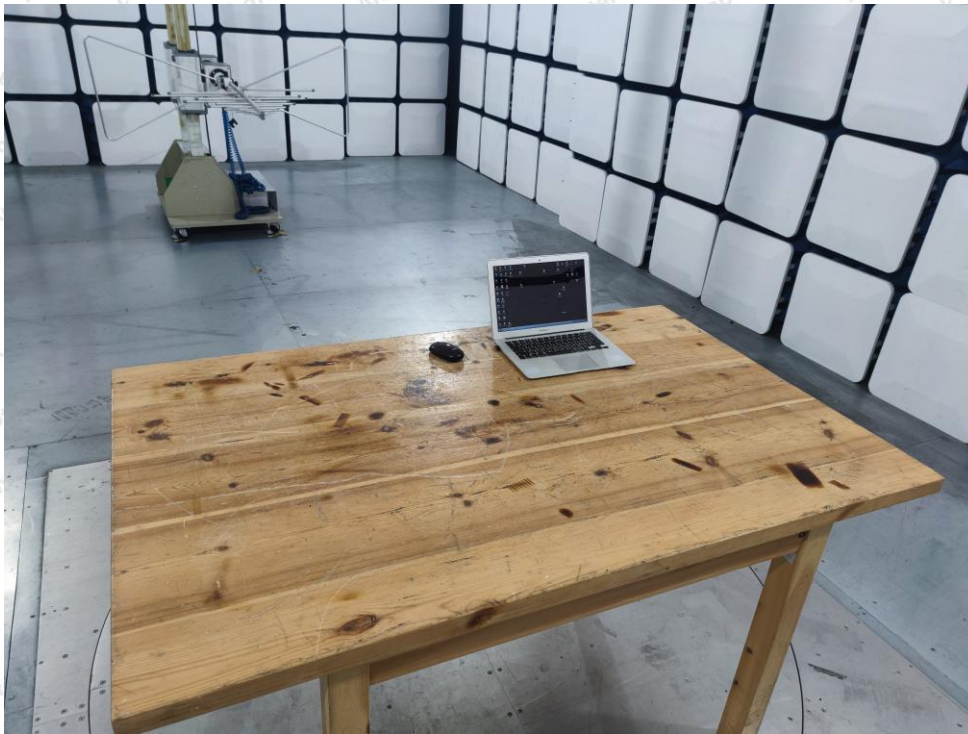
Photo of Radiation Emission Test
